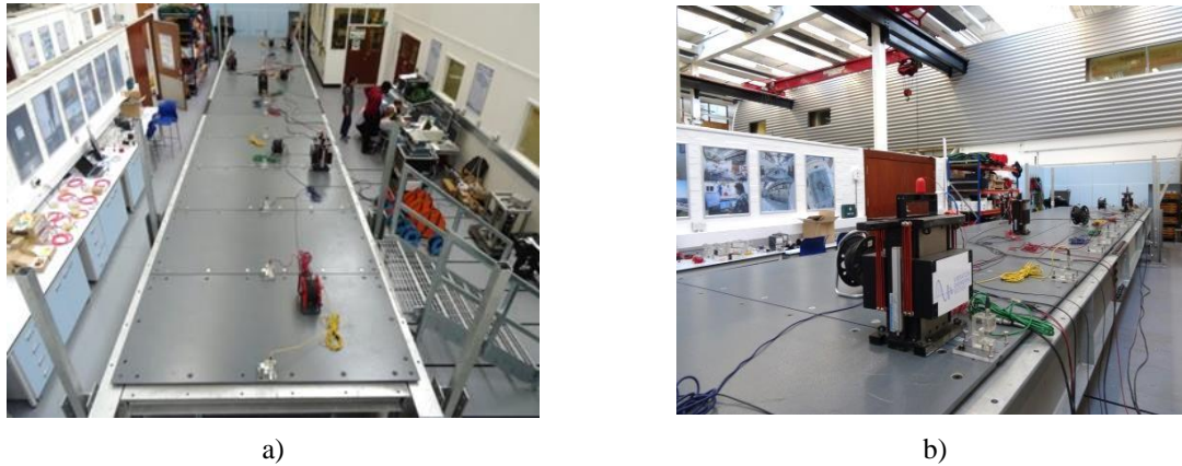
Figure 4.4. Laboratory footbridge: a) view on the footbridge; and b) Proof mass actuators APS Dynamics model 400 [124]
