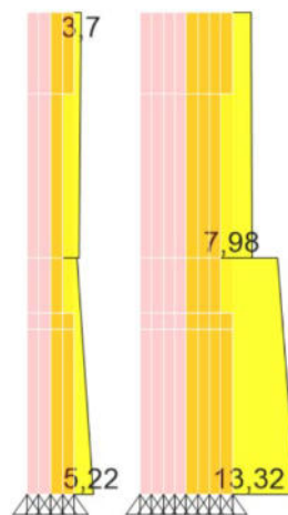
Elevation View - 3 Shear Force 2-2 Diagram (3. Komb) [kN]
