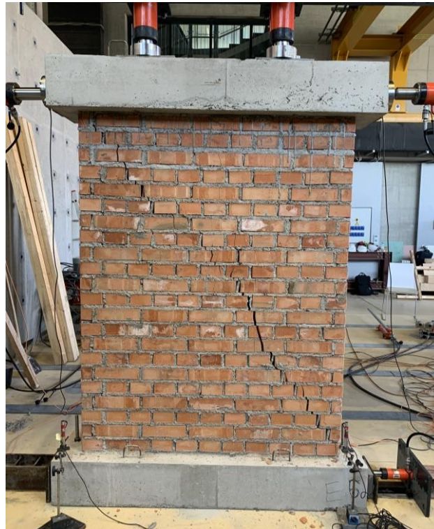
Figure 4.24 Final failure mechanism of URM 1 pier
