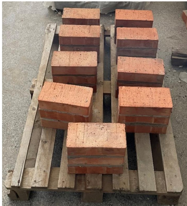
Figure 4.12 Nine test specimens for the initial shear strength test of masonry
