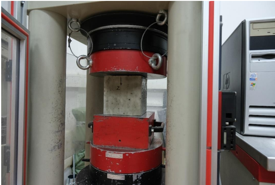
Figure 4.8 Compression strength testing of concrete cubes
