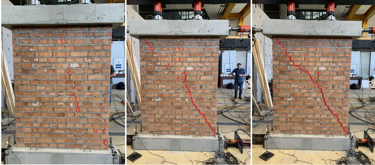
Figure 4.23 URM 1 a) Crack propagation - step 7 b) Crack propagation step - 10 c) Crack propagation - failure
