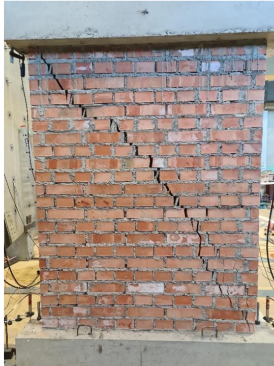
Figure 4.55 Final failure mechanism of CFRCM 1 pier
