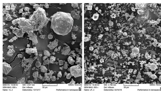
**Figure 3. Micrographs of WBA and coal fly ash (magnification SEM\_MAG = 800x)**
