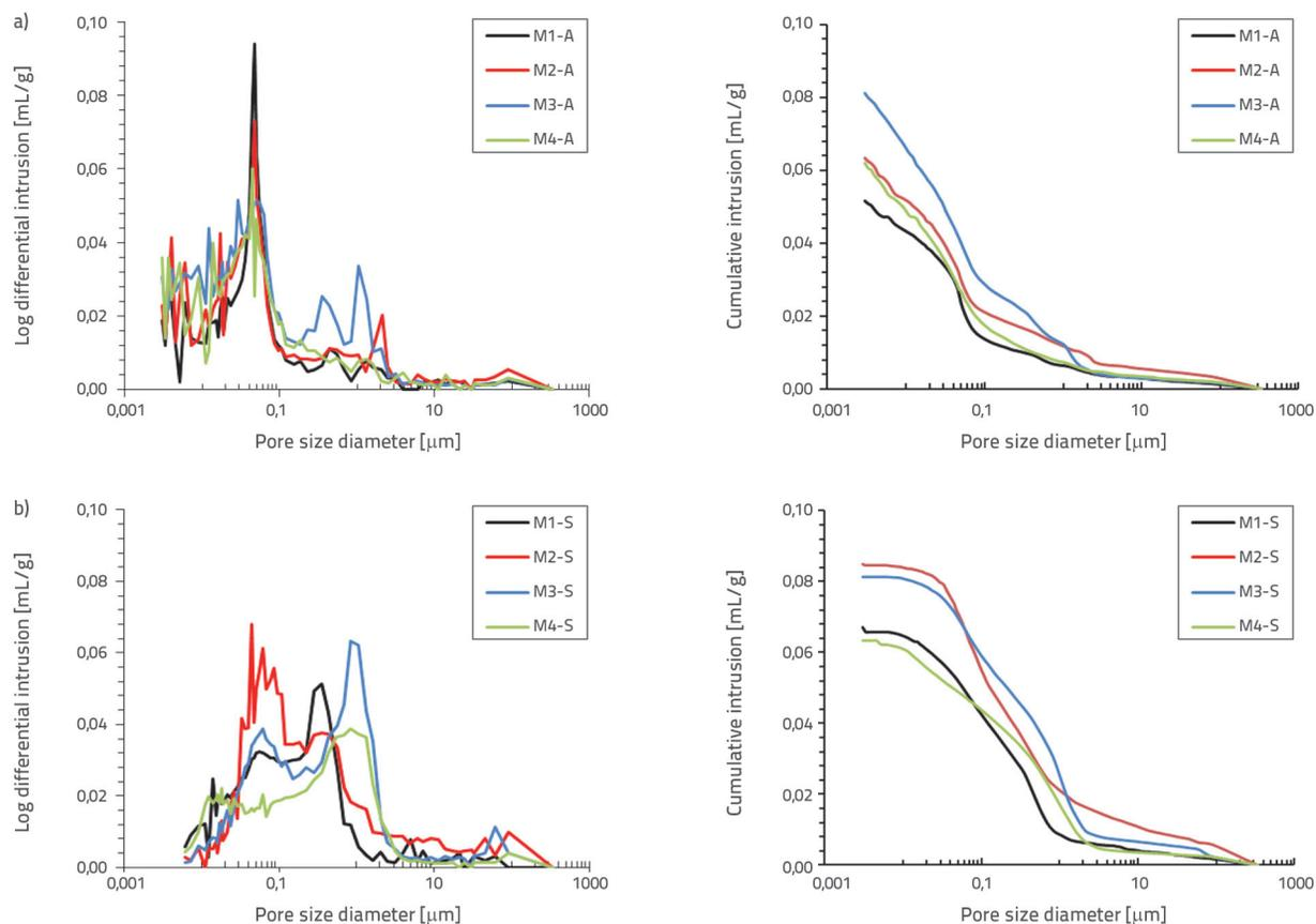
Figure 8. Differential pore size distribution (left) and cumulative pore size distribution (right) of: a) mortars samples cured at an RH of 95% and a temperature of  $20 \pm 2$  °C and b) mortars samples cured at an RH of  $60 \pm 10\%$  and temperature of  $21 \pm 2$  °C
