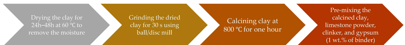
Figure 2. Steps involved in the preparation of LC3 in the lab for this study.
