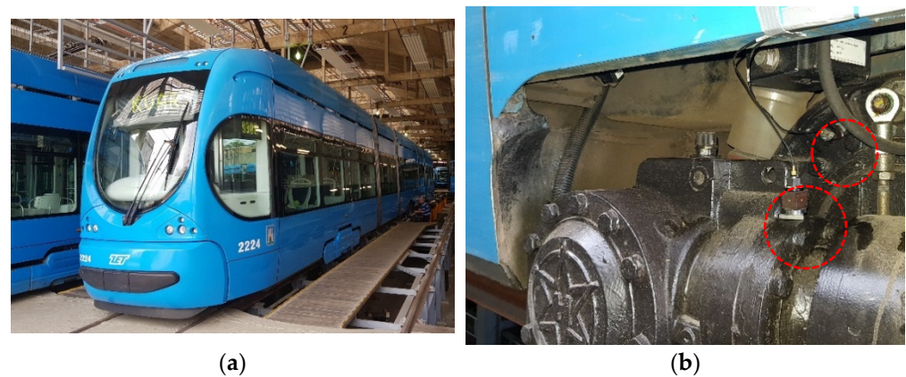
Figure 5. (a) Tram TMK2224 in the position for accelerometer mounting; (b) vertical and transverse accelerometers at the central bogie.
