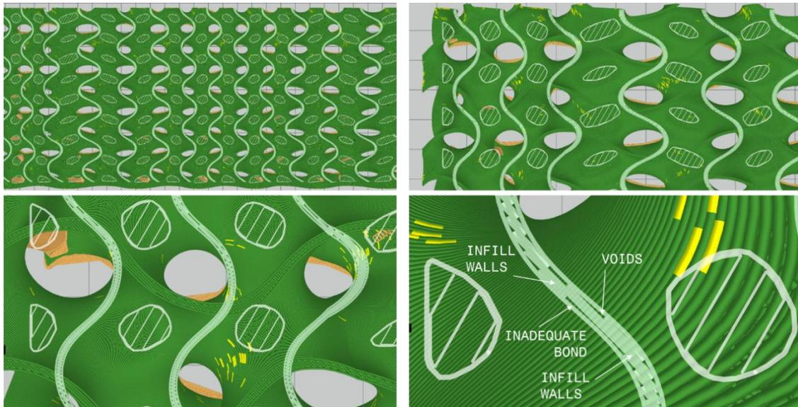
Figure 8.6 3D printing toolpath from GrabCAD slicer
