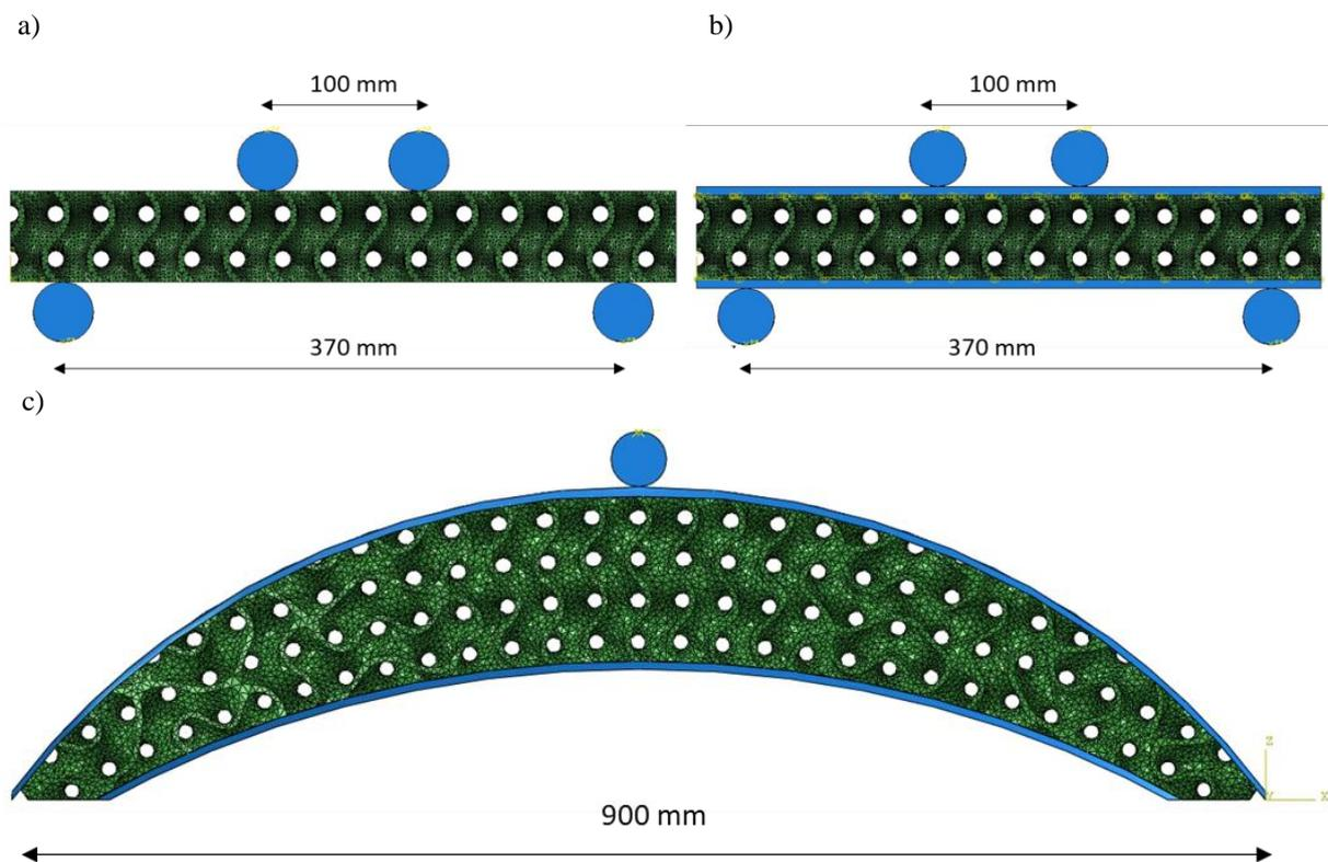
Figure 7.3 Finite element models: a) Core only; b) Sandwich beam; c) Arch beam
