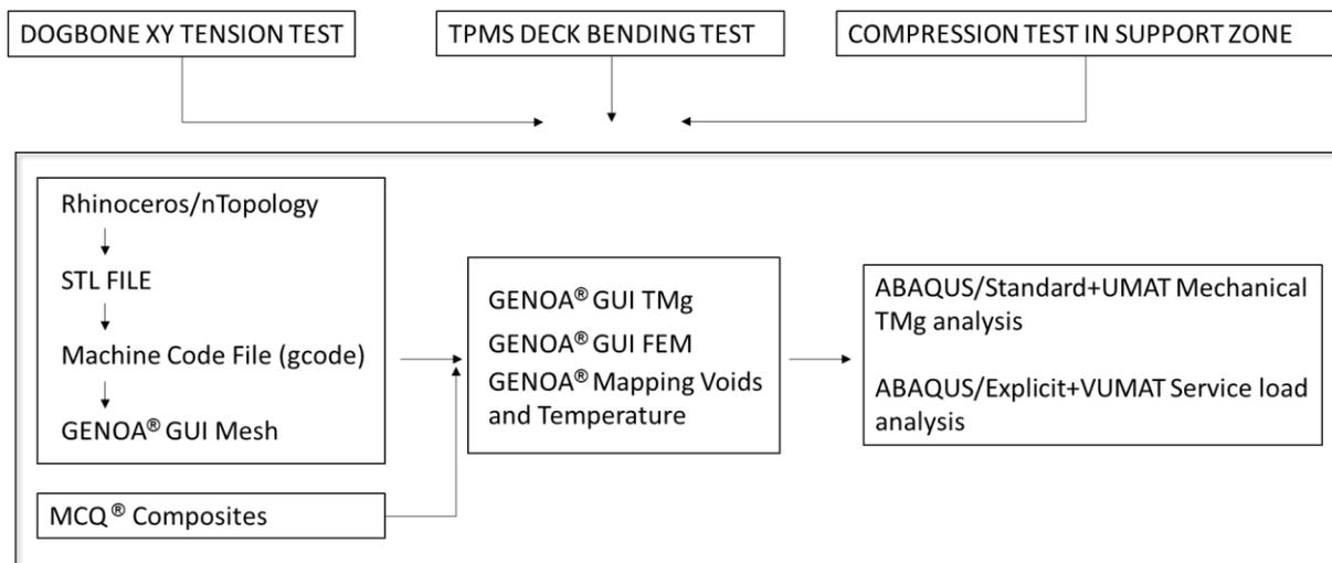
Figure 5.12 Flowchart of simulation approach
