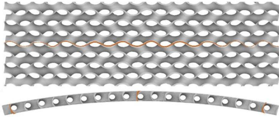
Figure 2.6: Topology optimization with Gyroid structure
