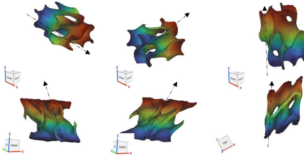
Figure 5.2 RVE Homogenization analysis set of 6 load cases
