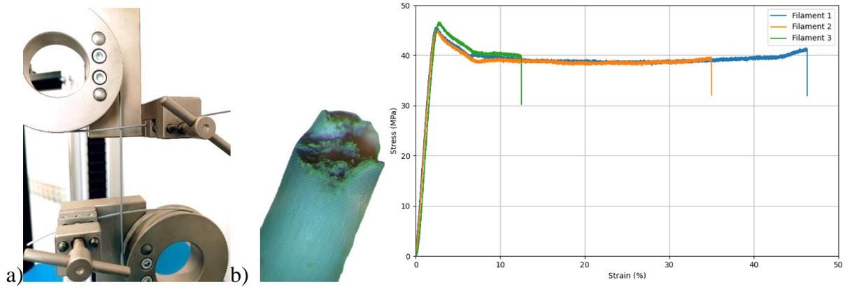
Figure 5.13: a) ASA filament tension test setup; b) Microscopic view of the fracture zone; c) stress-strain relationship obtained from the tensile test performed on the ASA filament specimen
