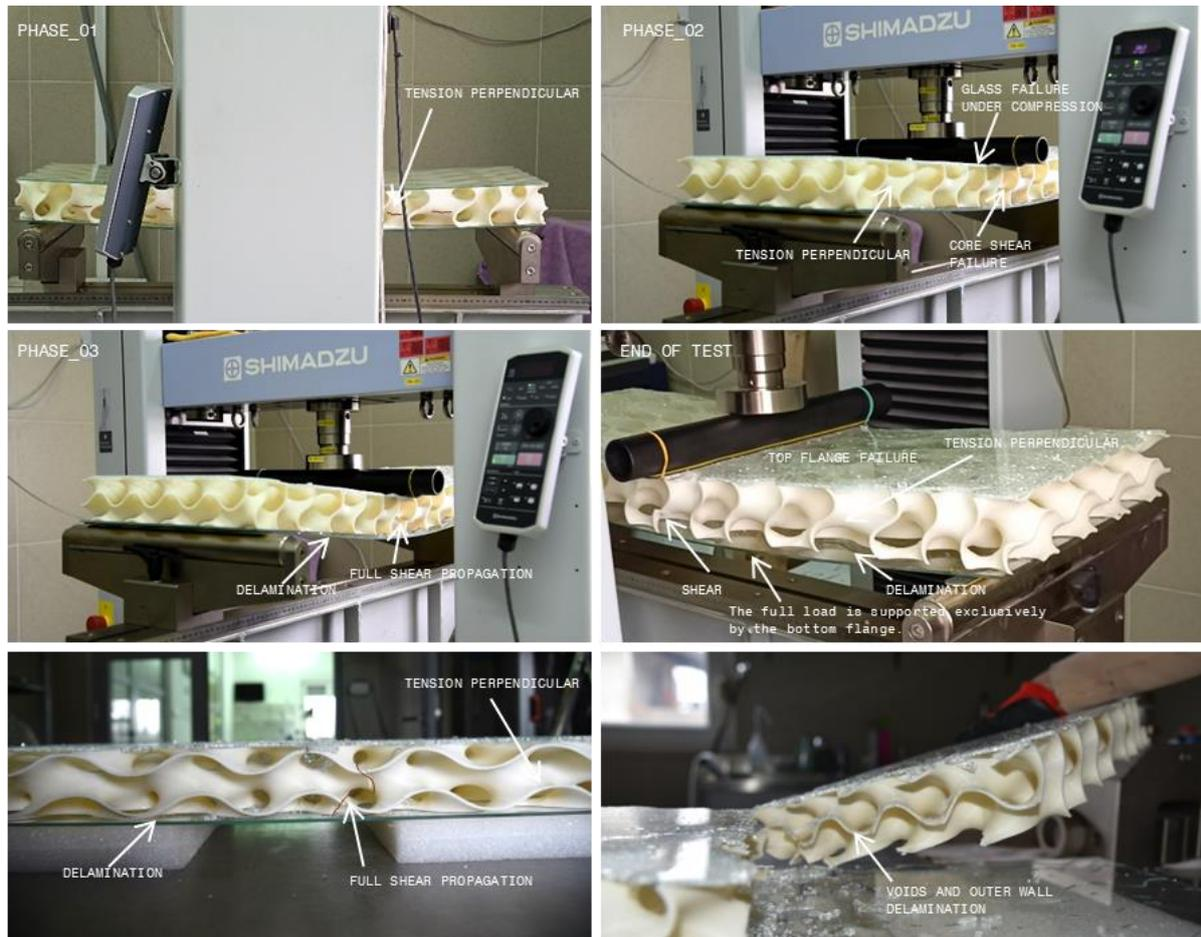
Figure 8.7 Snapshots from bending test by phases
