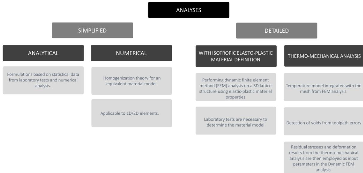
Figure 5.1 Analysis approaches from simplified to more detailed
