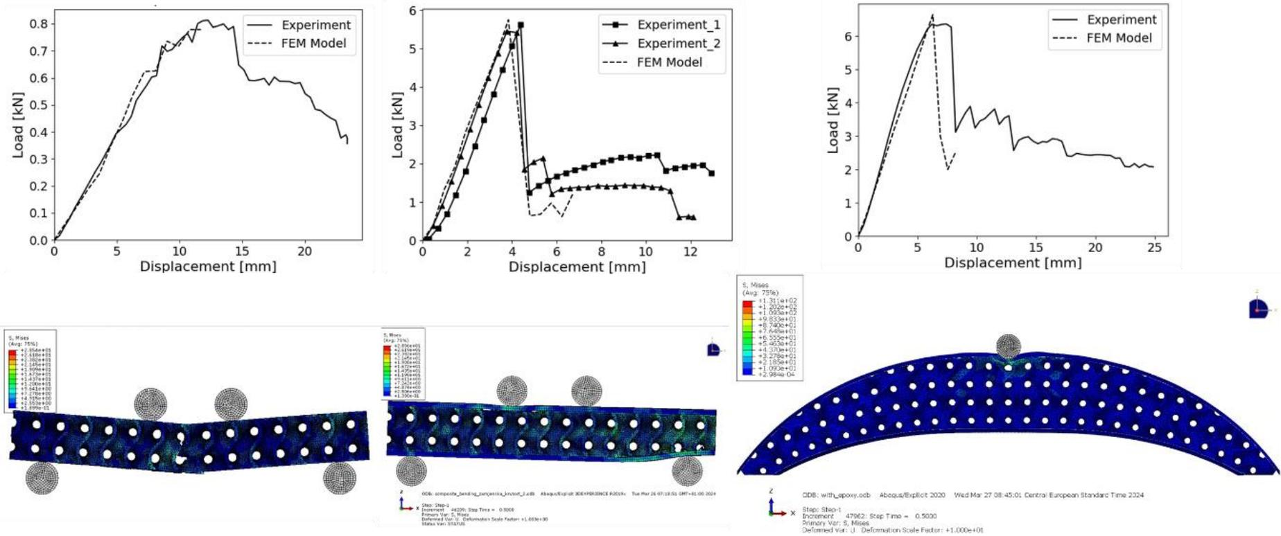
Figure 8.18 Comparison of load vs. displacement: FEM and experimental data for “core-only”, “sandwich beam”, and “arch beam”
