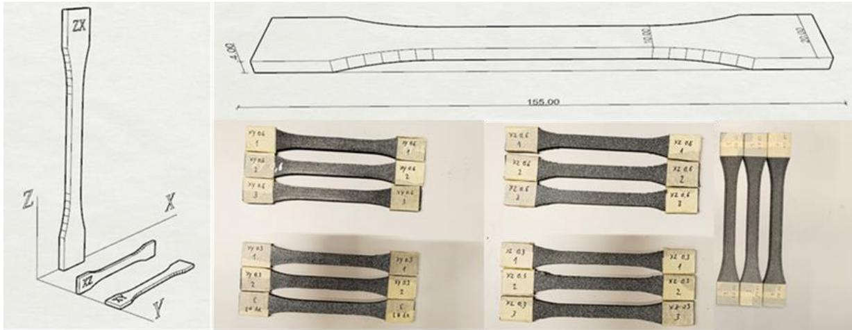
Figure 3.6 Tensile test specimens - HI\_TEMP CF material
