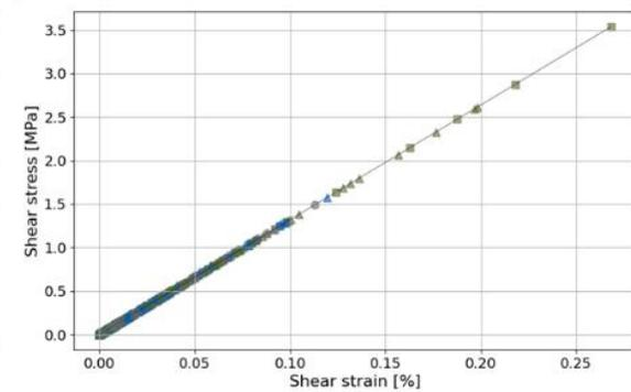
Figure 8.16 Arch beam: Shear stress vs. strain
