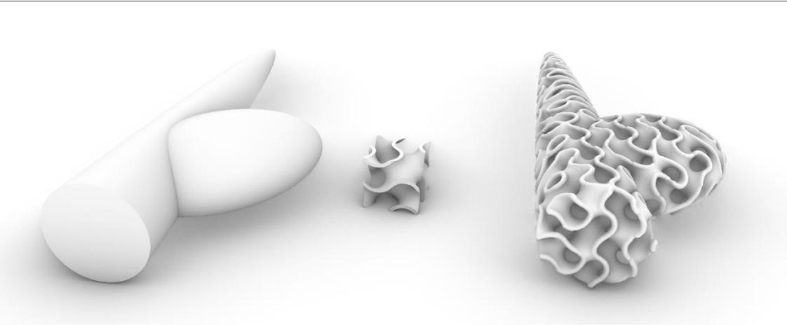
Figure 1.4 From 3D solid to porous TPMS structure
