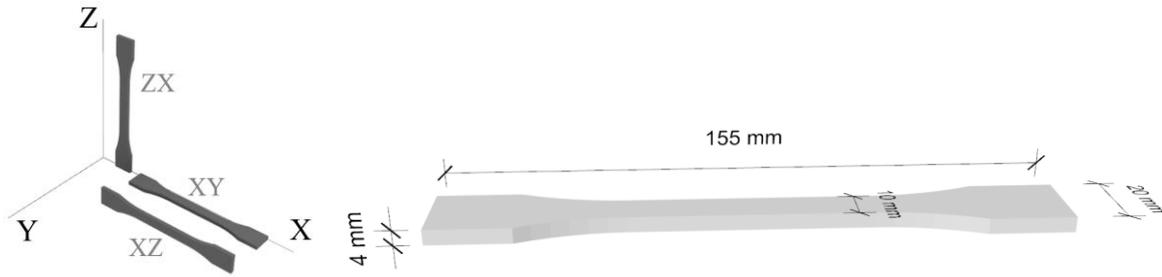
Figure 3.1: Dogbone ASA specimens for the tensile test
