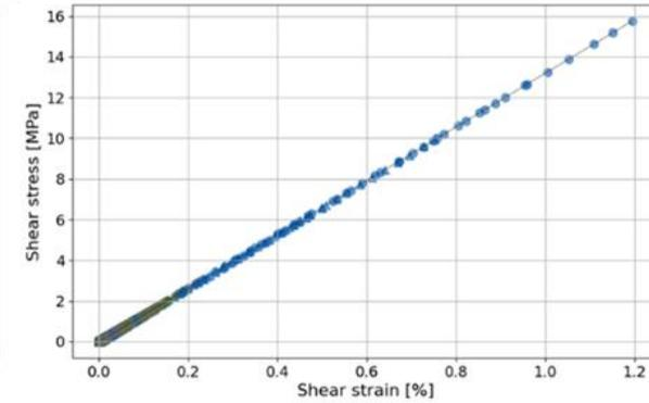
Figure 8.10 Core only: Shear stress vs. strain
