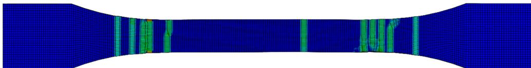
Figure 5.17 Strain concentration and potential fracture zones
