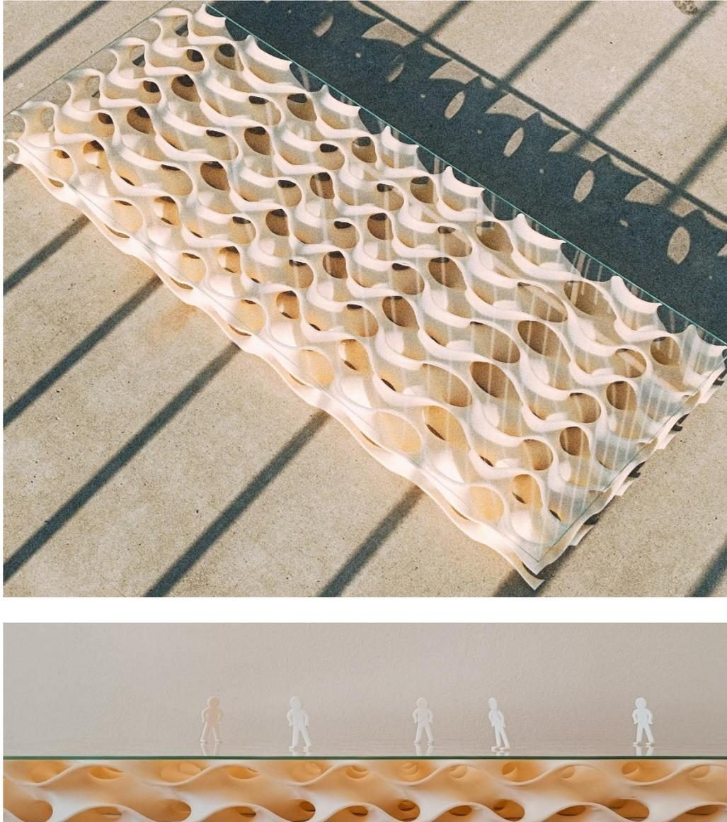
Figure 4.4 Final part of the composite TPMS bridge deck with tempered glass face sheets
