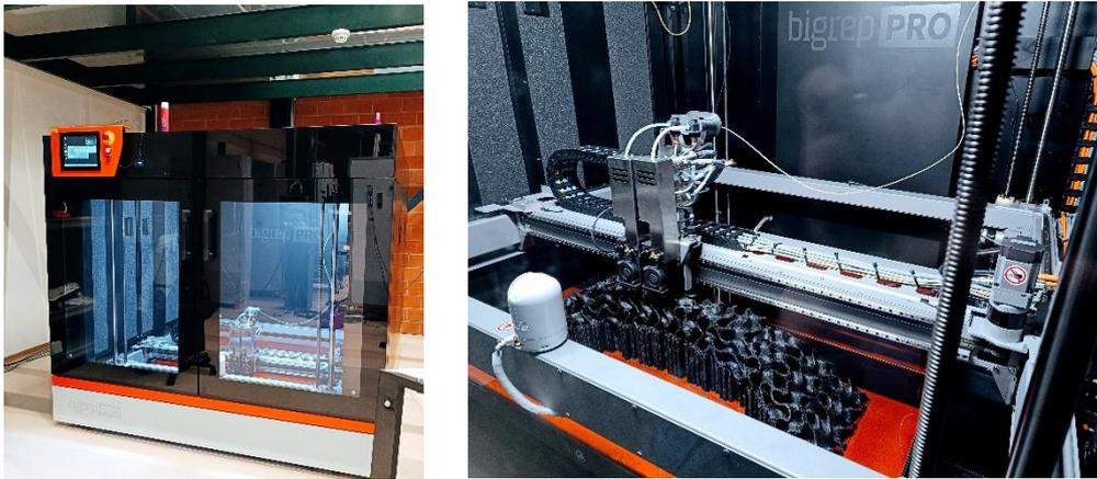
Figure 6.5 Bigrep PRO printer built print space of 1005 x 1005 x 1005 mm.
