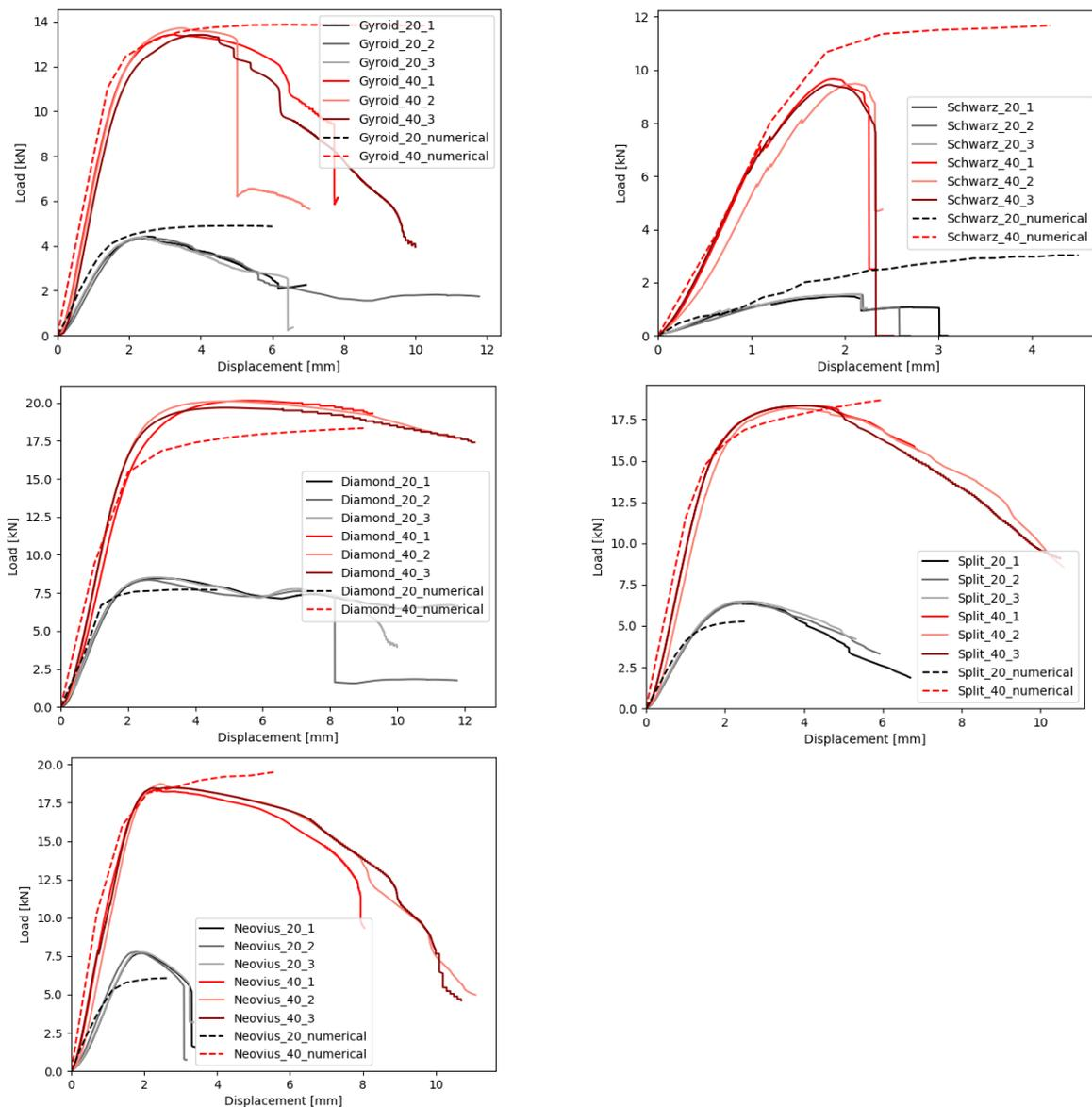
Figure 8.4 Compressive load-displacement diagrams for five TPMS geometries
