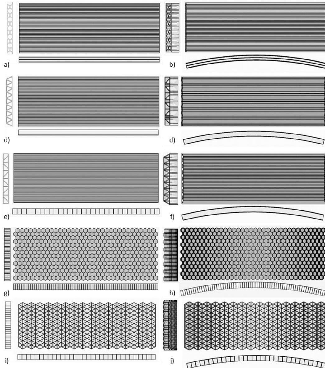
Figure 2.1 GFRP plate, adhesively bonded pultruded profiles: **(a)** Superdeck; **(b)** Superdeck in an arch; **(c)** EZSpan; **(d)** EZSpan in an arch; **(e)** DuraSpan; **(f)** DuraSpan in an arch; **(g)** Strongwell; **(h)** Strongwell in an arch. Sandwich panels: **(i)** triangular-shaped infill; **(j)** triangular-shaped infill in an arch; **(k)** honeycomb-shaped infill; **(l)** honeycomb-shaped infill in an arch.
