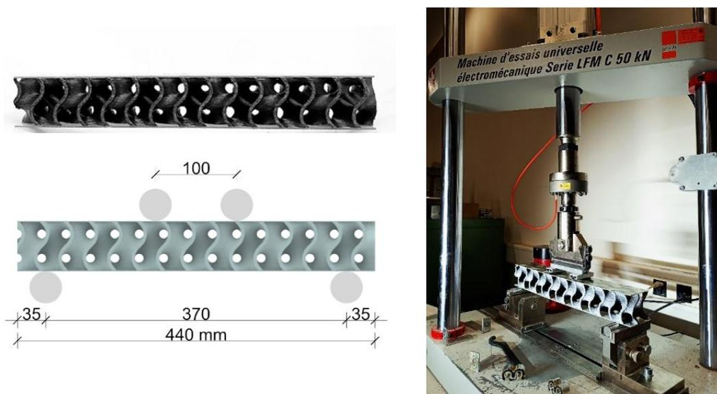
Figure 6.4 4-point bending test of beam samples
