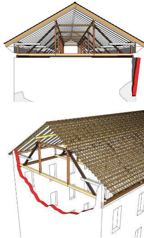
Figure 3: Typical damages to masonry walls
