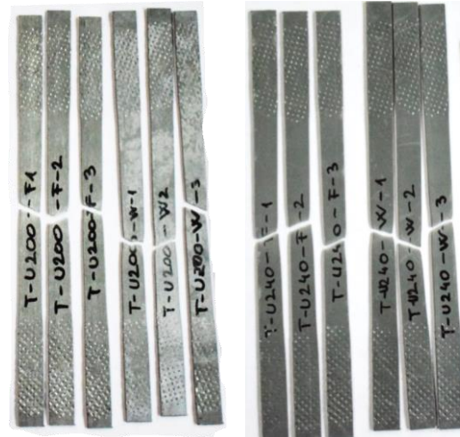
Figure 8: Tensile specimens after the test
