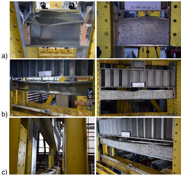
Figure 23: Deformations for 2C-SW-240-2.0 a) Local, b) Distortional, c) Interactive buckling
