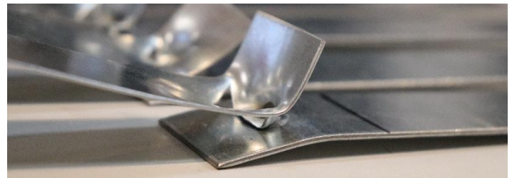
Figure 6: Full button pull-out failure mode of the spot welds
