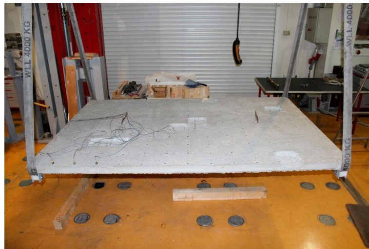
Figure 2. Suspended plate with discrete damages.
