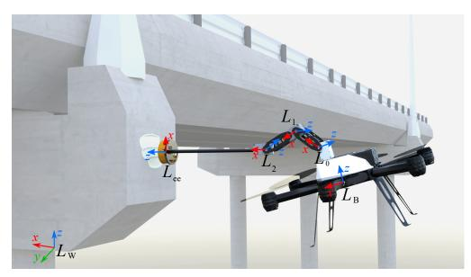
Figure 2. Coordinate systems of the world, UAV and the 3-DoF manipulator.
