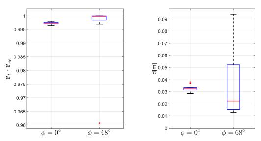
Figure 12. (Left): box and whiskers plot of the dot product between the blob plane normal vector  $\mathbf{r}_{t}$  and the end-effector orientation vector  $\mathbf{r}_{ee}$ ; and (Right): box and whiskers plot of the distance from the target point after contact.
