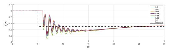
**Figure 9.** Force response comparison for different values of the parameter  $\beta$ . The analysis was conducted on a plane perpendicular to the ground where the force reference along the x axis is required.
