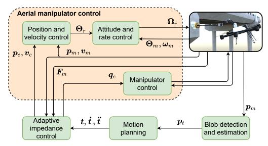
**Figure 4.** The overall functional schematic of the system. The aerial manipulator control subsystem is necessary for the controlling position and attitude of the UAV, and manipulator joints. On top of this controller, the adaptive impedance control is employed in order to track the desired force. Motion planning generates an appropriate trajectory based on the target point supplied by the blob detection algorithm.
