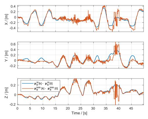
**Figure 7.** This figure shows the comparison of normalized motion of the UAV body frame as observed from the Optitrack world frame and as observed from the detected blob frame labeled  $\mathbf{p}_B^W[k] - \mathbf{p}_B^W[0]$  and  $\mathbf{p}_B^{blob}[k] - \mathbf{p}_B^{blob}[0]$ , respectively.
