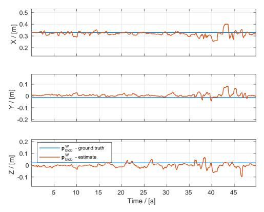
**Figure 8.** This figure shows the comparison of the ground truth blob position and the blob position estimate expressed in the Optitrack world frame. The root mean squared error across all three axes is 4.6 cm.
