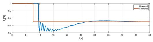
**Figure 10.** Force response in case of a contact plane perpendicular to the ground,  $\delta = 0^{\circ}$ .
