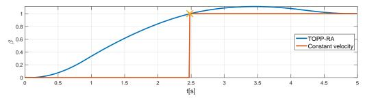
**Figure 5.** Visual comparison between TOPP-RA and the piecewise constant velocity interpolation. Waypoints for both trajectories are kept the same, and around t = 2.5 s, the middle waypoint(yellow cross) is reached. Although the dynamical constraints are the same, TOPP-RA takes other degrees of freedom into account and produces a trajectory with overshoot which is not suitable for parameter  $\beta$ .
