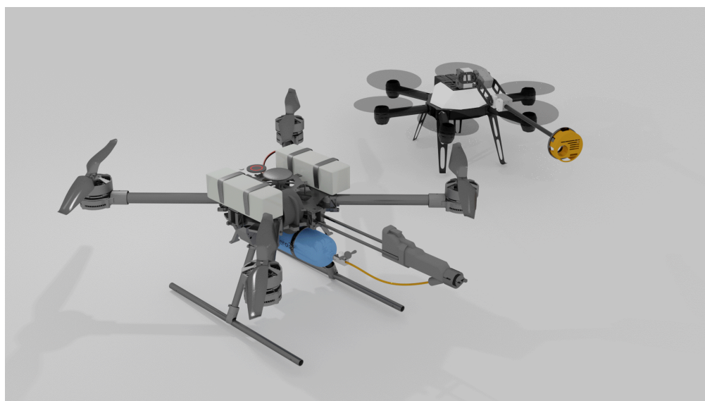
Figure 1. Two aerial robots working together to attach sensors to different parts of a bridge and similar grade separation infrastructure. The one on the left is used to spray the resin onto the surface, while the aerial robot on the right maintains contact to the surface with the sensor attached to its end-effector.
