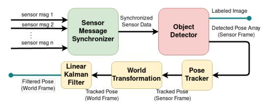
**Figure 6.** The pipeline for the modular object detection framework. Inputs to the system are an arbitrary number of sensor messages (image, depth, point cloud, etc.) along with sensor–world frame transformations. Output is the detected blob pose in the world frame. The synchronizer and detector are modular components, while the linear Kalman filter, world transformation and pose tracker stay invariant.
