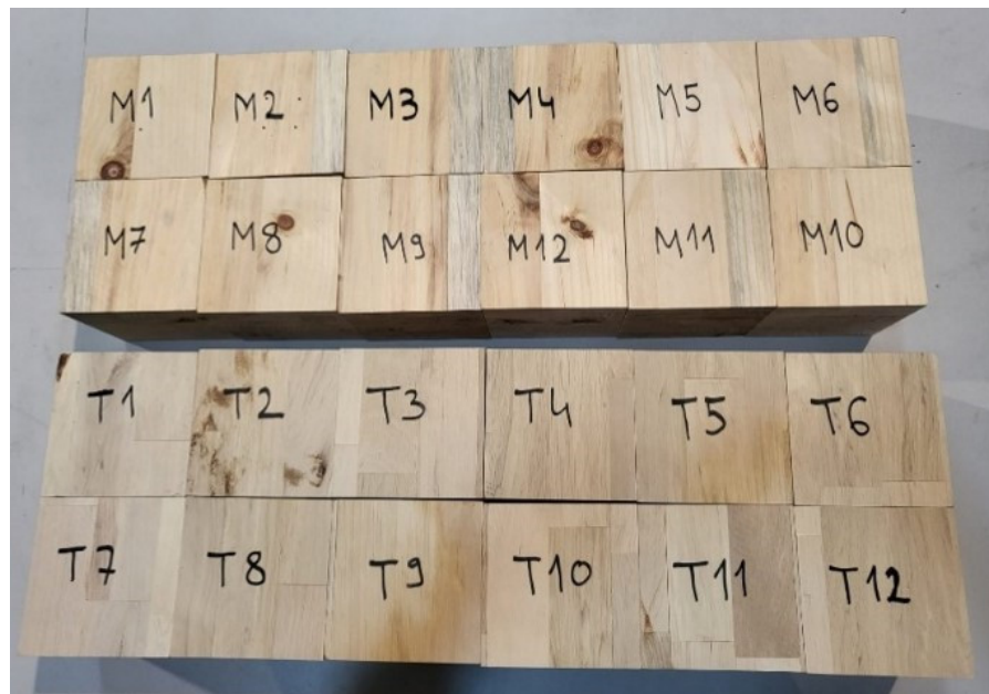
Figure 4. Cube specimens—density measurement.
