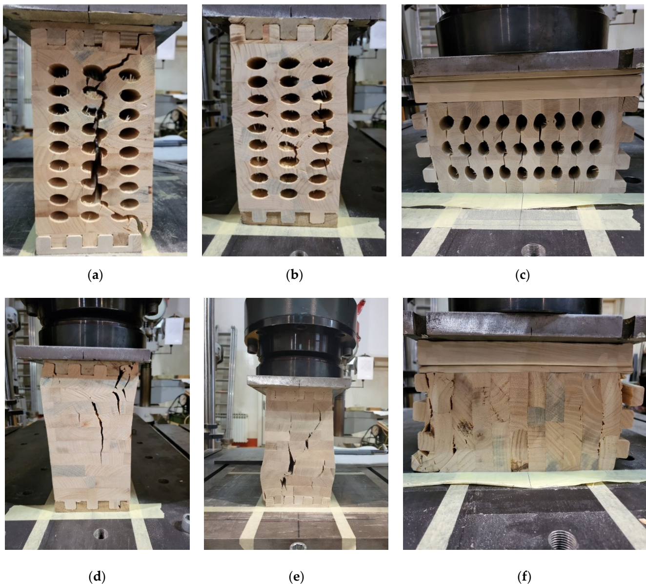
Figure 10. Failure modes characteristic for group of specimens: (a) ME-209 mm; (b) TE-209 mm; (c) ME-400 mm; (d) MP-209 mm; (e) TP-209 mm; (f) MP-400 mm.
