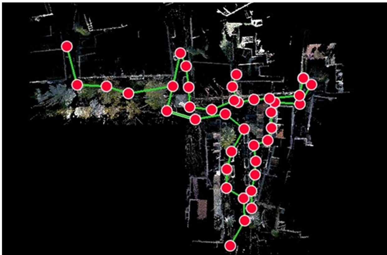
**Figure 9.** Plan view of the point cloud showing camera stations.
