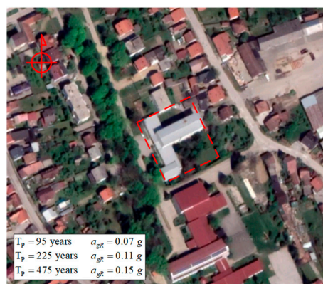
Figure 10. Horizontal peak ground accelerations for soil class A at the location [Google maps].
