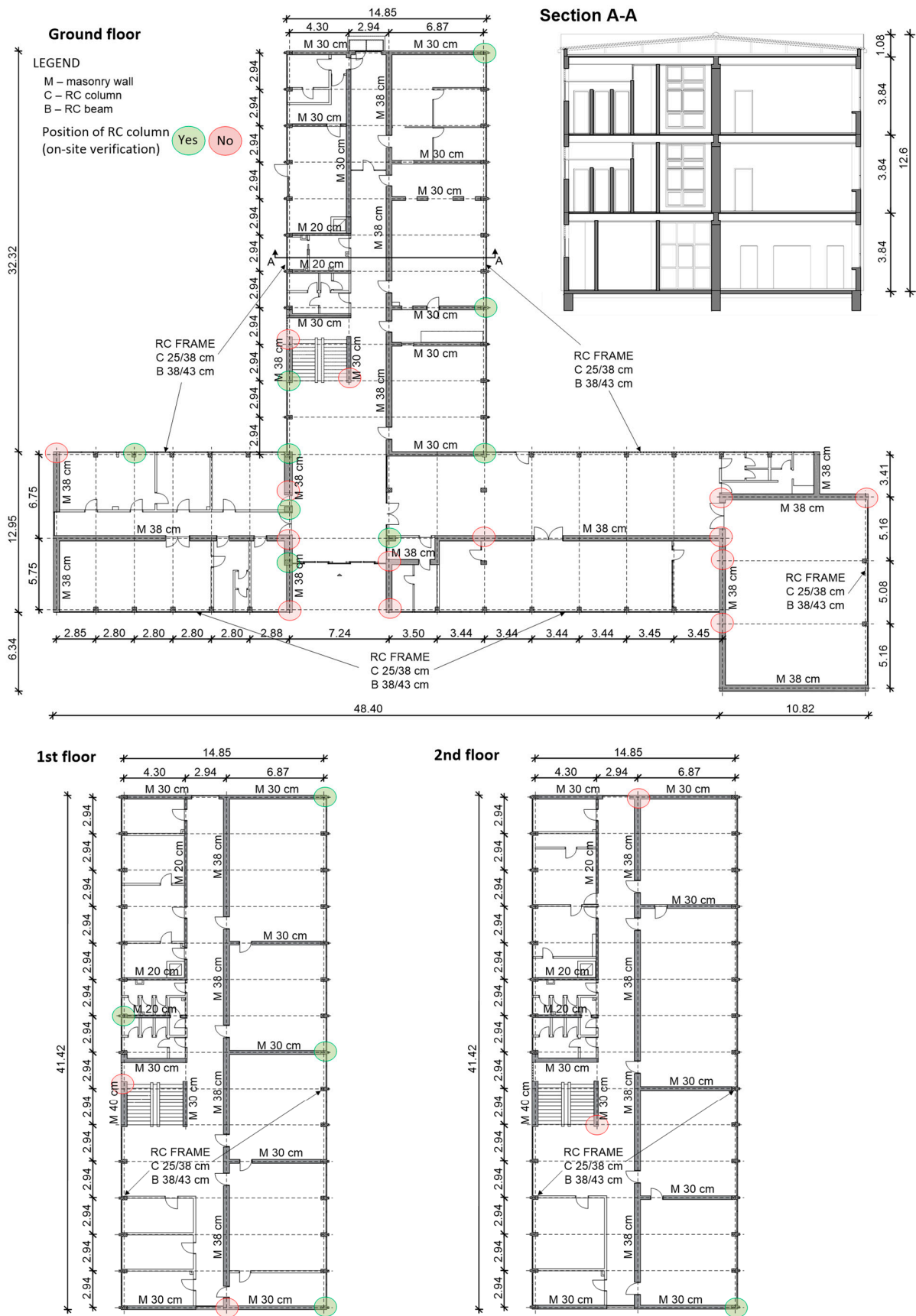
Figure 5. Layout of the building stories and markings of gravity and lateral load resisting system dimensions.
