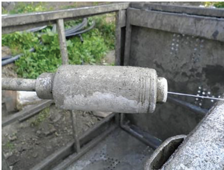
Fig. 5: Roto nozzle for washing of concrete surface.
