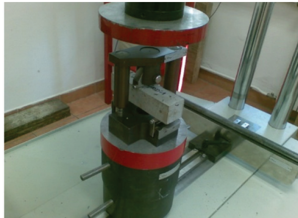
Fig. 7: Mortar samples for compressive and bending strength testing (left) and testing of bending strength (right).
