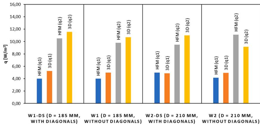
Fig. 19. Calculated heat flux densities for all methods.
