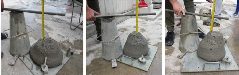
Fig. 6. Slump test for concrete with air entrainment: (a) without fibers, (b) with 0.9 kg/m<sup>3</sup> of RTPF, and (c) with 1.8 kg/m<sup>3</sup> of RTPF.
