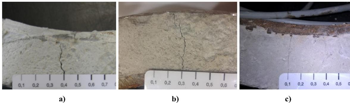
Fig. 15. Crack width obtained by visual inspection for mixes: (a) without fibers, (b) with 0.9 kg/m<sup>3</sup> of PP, and (c) with 0.9 kg/m<sup>3</sup> of RTPF.
