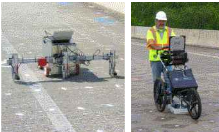
Figure 3 Delamination detection using IE (left) and GPR survey (right).
