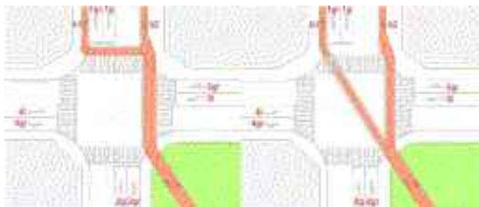
Figure 9 Diagram of two-step crossing (left) vs. diagonal layout (right).
