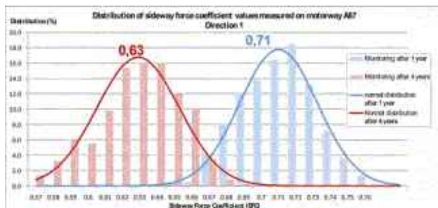
Figure 3 Evolution of skid resistance on motorway A87 – Direction 1
