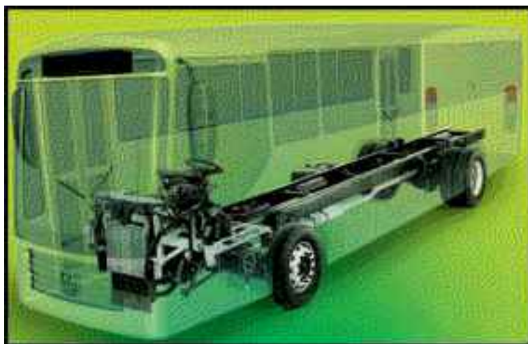
Figure 1 Typical front engine bus configuration [1]
