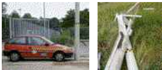
a) The vehicle and the column before crash test b) The column after the impact – vehicle speed was reduced to 60 km/h
