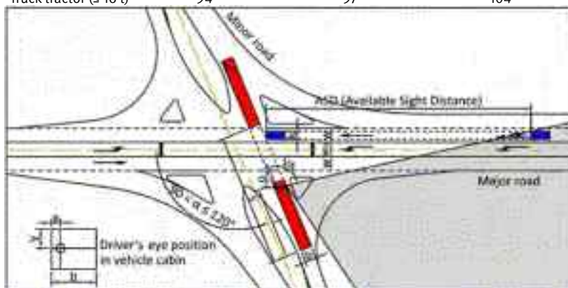
Figure 2 The scheme of the intersection for the calculation of available sight distance (ASD)
