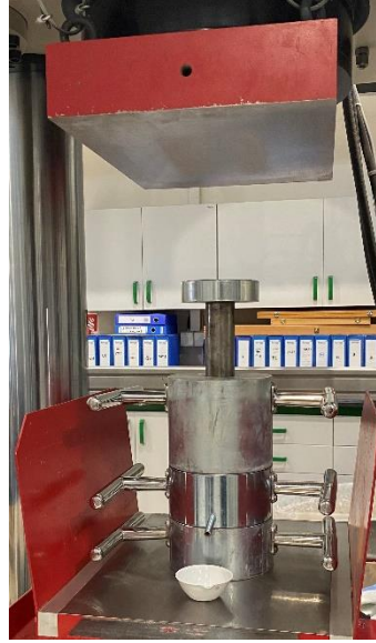
Figure 4.7 High pressure machine to extract pore solution.
