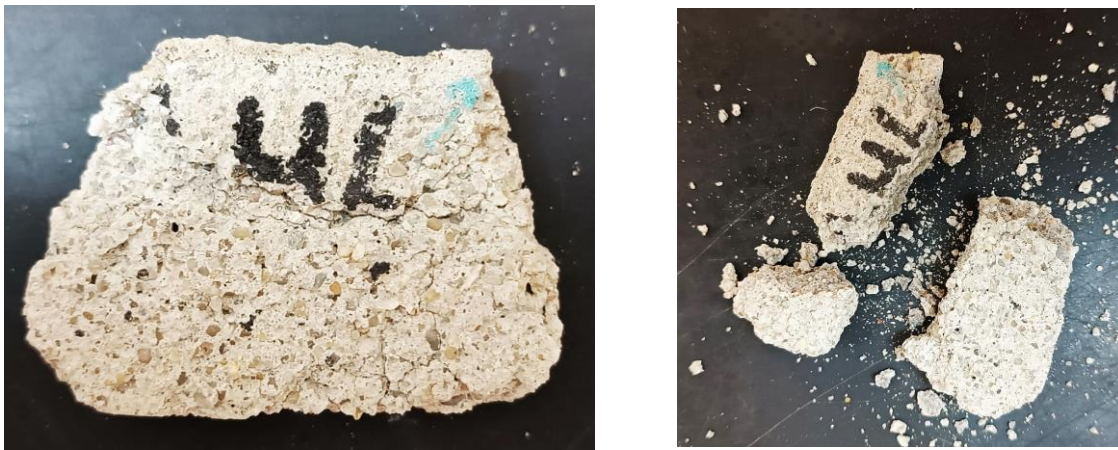
Figure 4.53. The AHL 5-40-M 'S2-c' specimen, displaying prominent degradation after enduring 14 cycles
