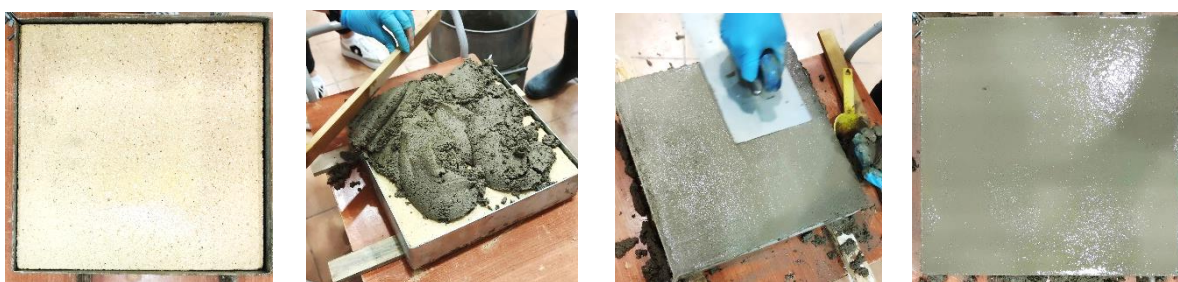
Figure 4.41. Coating of brick substrate with AHL mortar for pull-off testing
