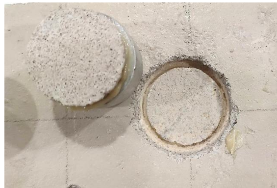
Figure 4.43. Failure of AHL 2-20-M mortar slab after pull-off test (delamination)
