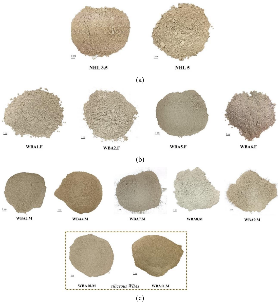
Figure 3.1. Powder samples of AHL raw materials: (a) primary NHL binders; (b) sieved fly WBAs and (c) sieved mixed WBAs, including siliceous variations
