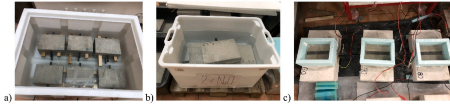
Fig. 2. The laboratory specimens: a) Group M , where various degrees of saturation are achieved by immersion in water, b) Group Cl , where various degrees of chloride concentration in the concrete cover are achieved by immersion in sodium chloride solutions, c) Group C , where various degrees of corrosion are achieved by exposure of the specimens to external current.
