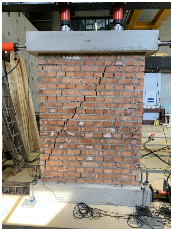
Figure 4.29 Final failure mechanism of URM 2 pier
