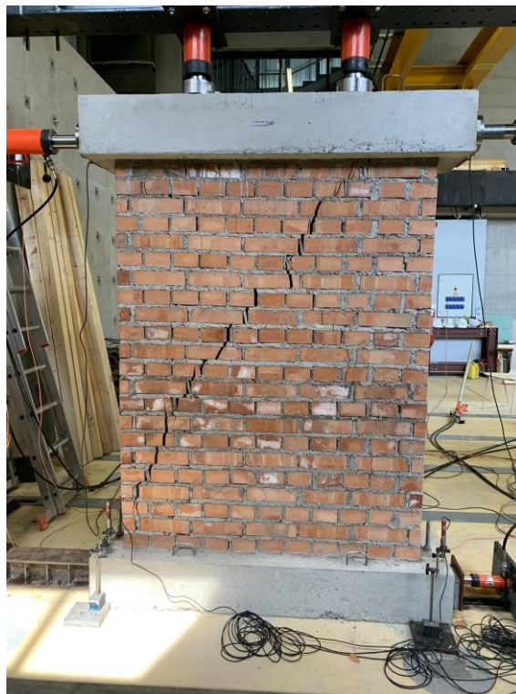
Figure 4.29 Final failure mechanism of URM 2 pier
