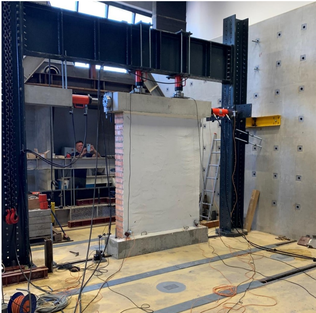
Figure 4.38 Testing of a FRCM pier
