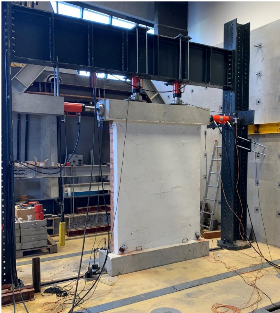
Figure 4.53 Testing of a CFRCM pier
