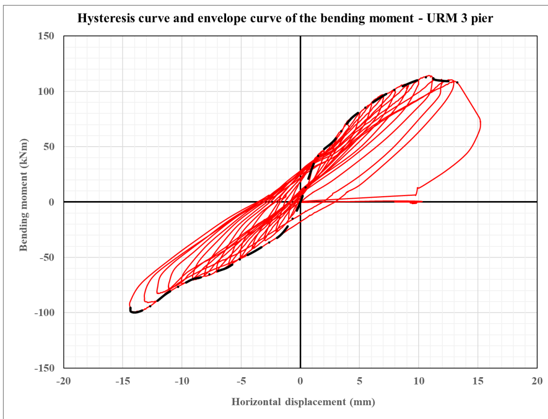
Figure 4.69 Hysteresis curve and envelope curve of the bending moment – URM 3 pier
