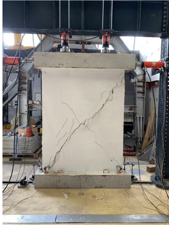
Figure 4.59 Final failure mechanism of CFRCM 2 pier
