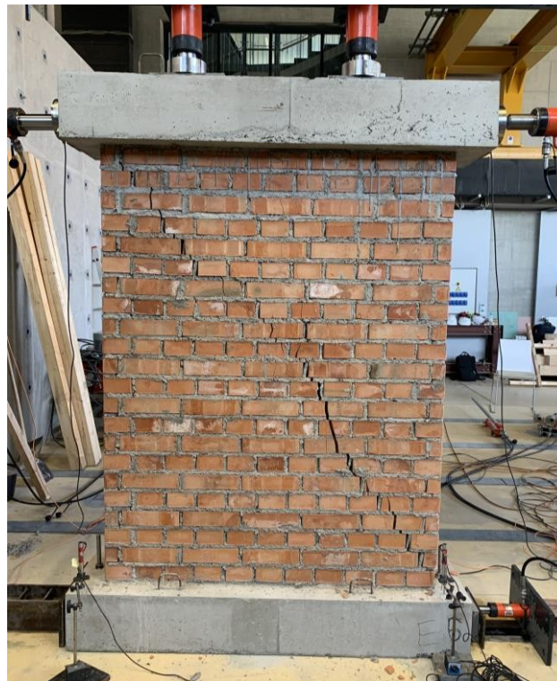
Figure 4.24 Final failure mechanism of URM 1 pier
