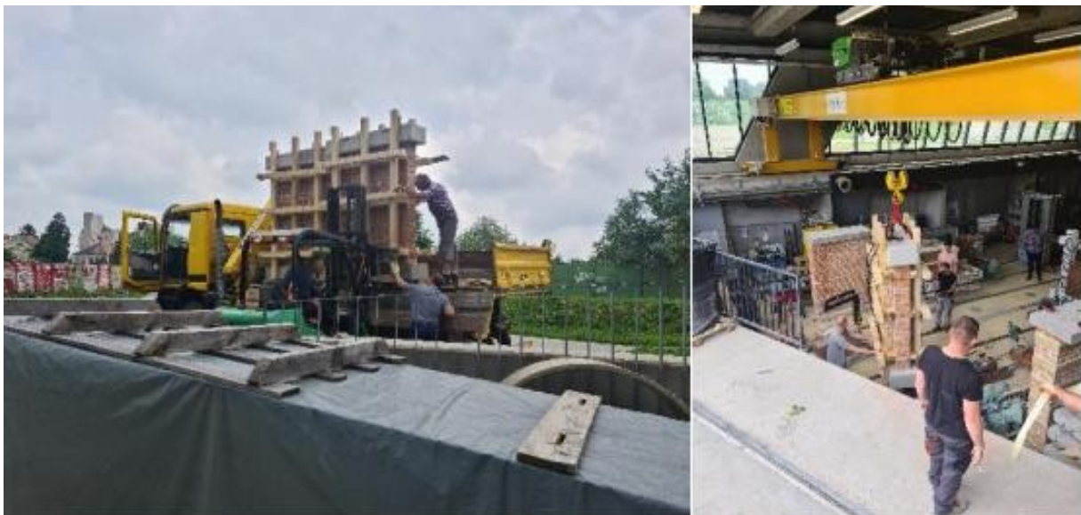
Figure 4.17 Transportation of masonry piers inside the laboratory
