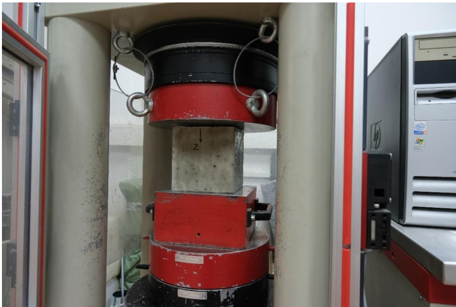
Figure 4.8 Compression strength testing of concrete cubes
