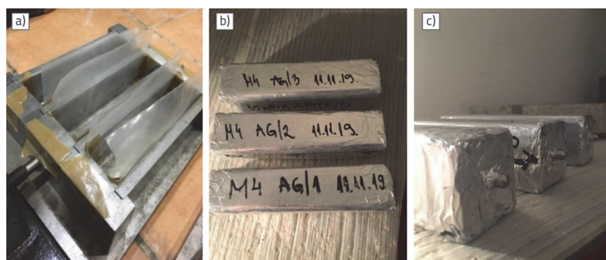
Figure 1. Testing of autogenous deformation: a) prepared mould; b) samples coated with aluminium foil; c) measuring rappers
