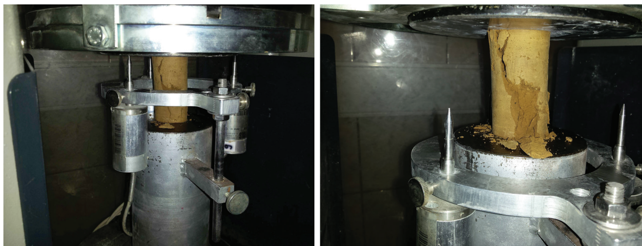
Figure 3. Testing compressive strength of composite in laboratory of Department of Geotechnics, Faculty of Civil Engineering, Zagreb
