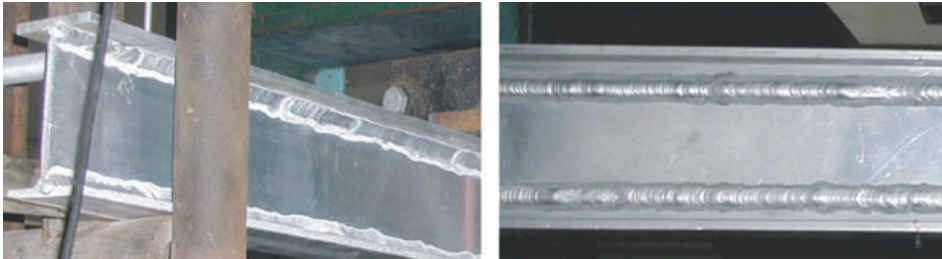
Figure 4. Longitudinally welded aluminium specimens: a) Type T cross-section; b) Type P cross-section [31]
