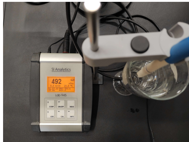
Figure 7. Measuring the electrical conductivity of water using the SI Analytics Lab 945 conductometer.
