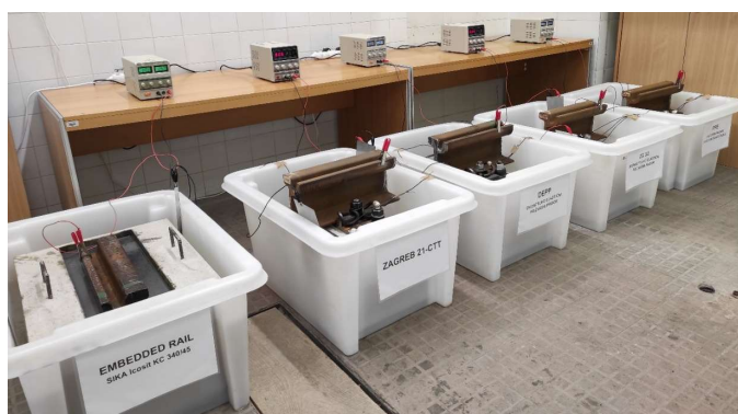
Figure 13. Samples before starting the experiment and electrical resistance measurement.
