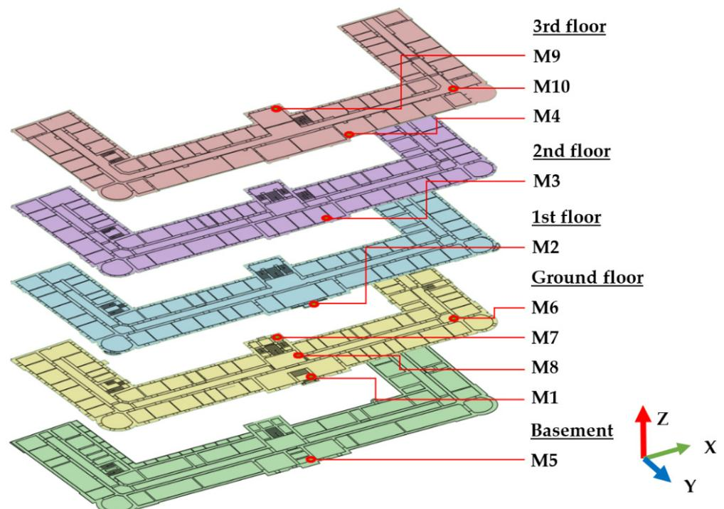
**Figure 6.** Layout of triaxial accelerometer measurement positions.
