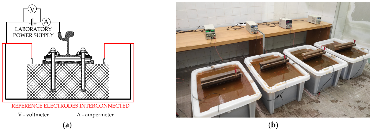
Figure 6. (a) Current circuit during testing and (b) samples during testing.
