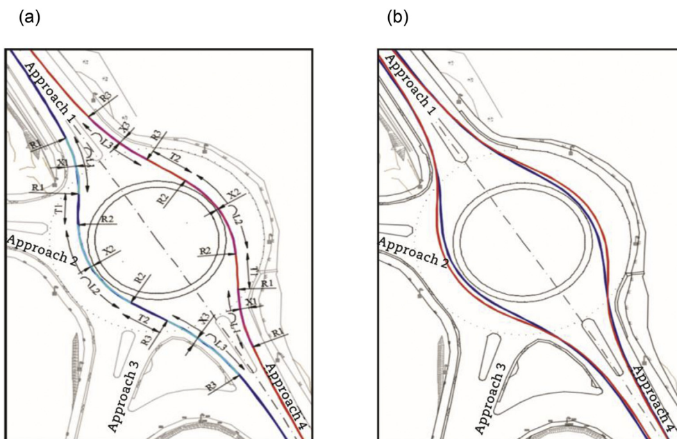
Fig. 11 – Theoretical and optional paths on roundabout A. (a) Elements of optional path. (b) Comparison of theoretical and optional paths.
