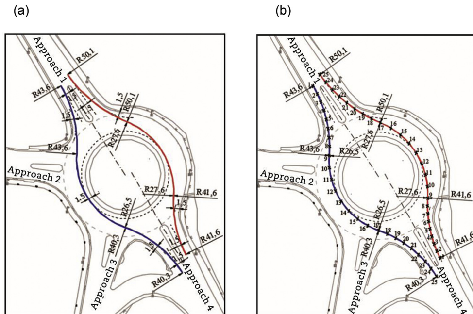
Fig. 7 – Theoretical path according to FHWA model and stakeout points for roundabout A. (a) Theoretical path. (b) Stakeout points.
