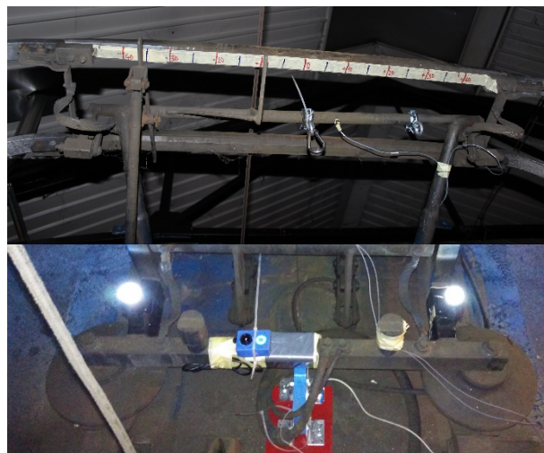
Fig. 7. Overhead wire stagger measurements using camera and measuring strip on the head and camera in the base.
