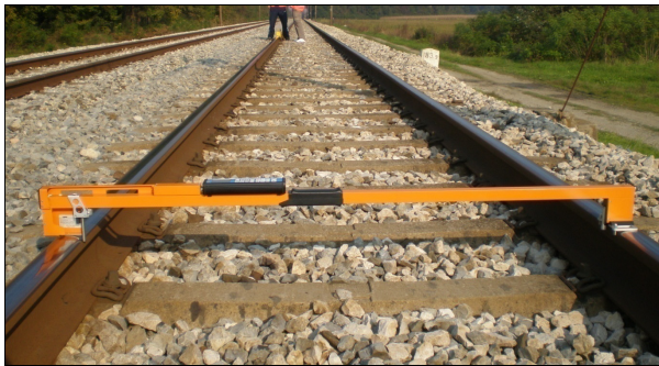
Figure 3 Manula track geometry measurement
