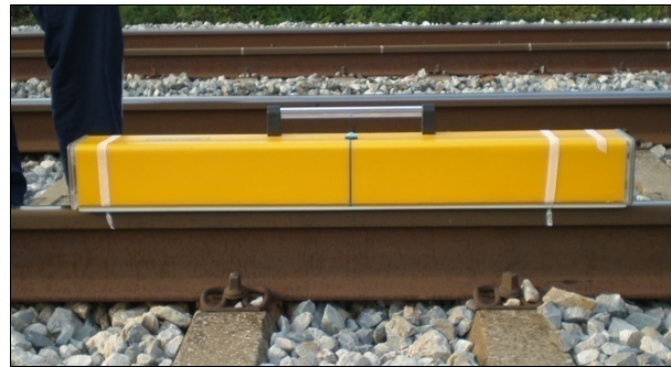
Figure 4 Rail surface roughness measurement
