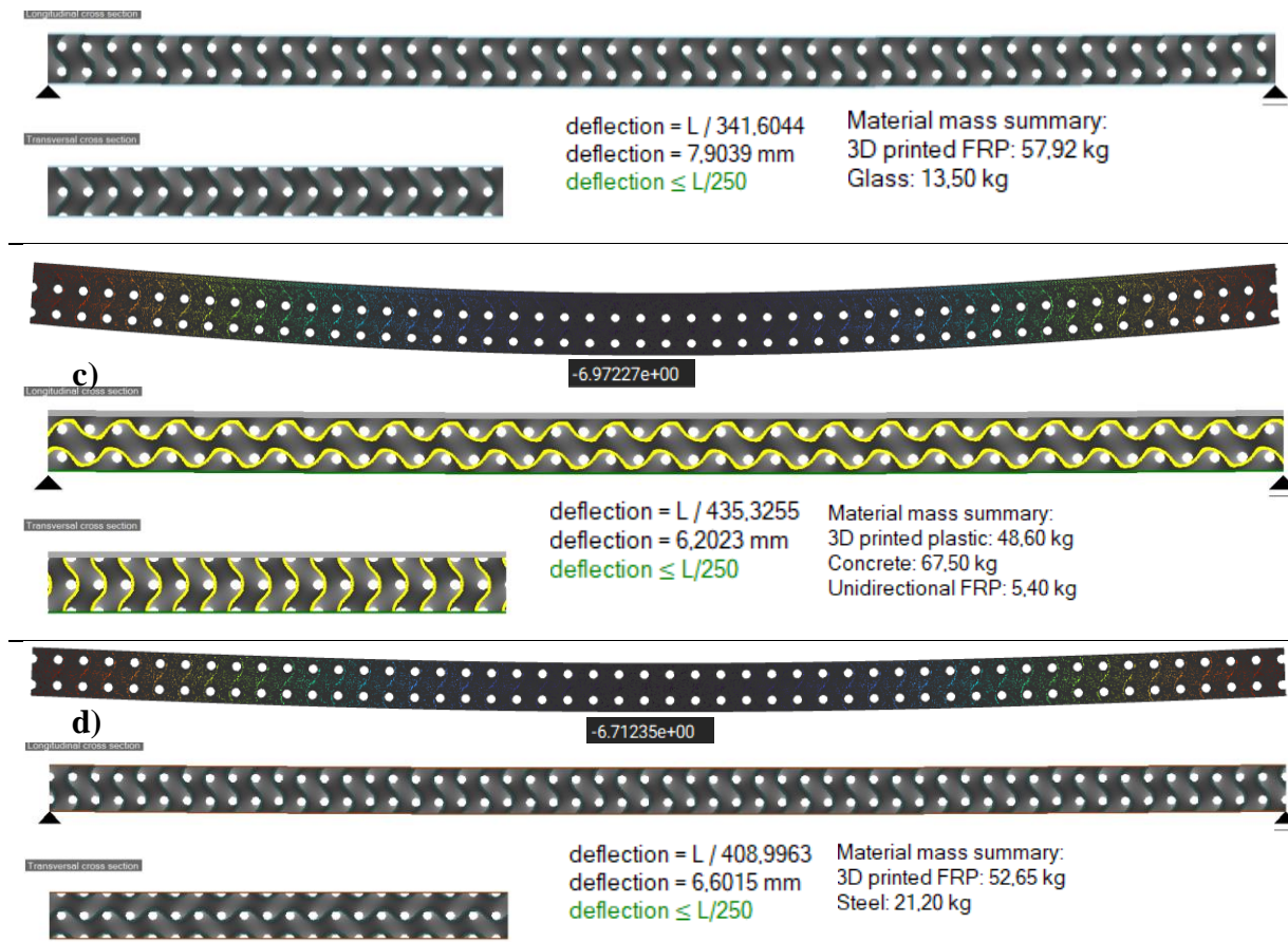
Figure 5.11 Optimised composite plate with 15% gyroid core - FEM and results from quick estimation algorithm: a) 200 mm core and top and bottom 10 mm flange from 3D printed unfilled plastic; b) 110 mm core from 3D printed filled plastic and 1 mm top and bottom glass flange; c) 120 mm core from 3D printed unfilled plastic, 10 mm top concrete and 1 mm bottom FRP flange; d) 100 mm core from 3D printed filled plastic and 0.5 mm top and bottom steel flange
