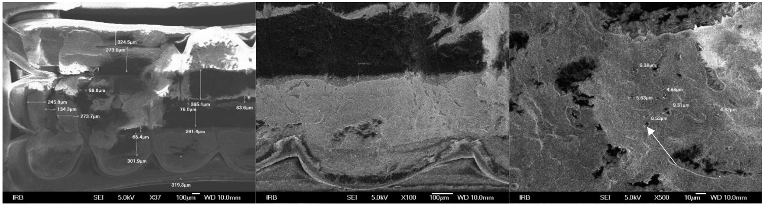
Figure 3.4 Scanning electron micrographs of (a) ASA XY print direction showing when a strut at 0^\circ direction is printed on a bottom 90^\circ direction strut (b) Printing in the XZ direction displays layers of elliptical shape in the cross-section, revealing irregularities and visible open cavities between 0 and 90^\circ c) The ASA ZX print orientation exhibits a localized thickening effect by placing a strut at a 0^\circ angle over a strut at a lower 90^\circ direction
