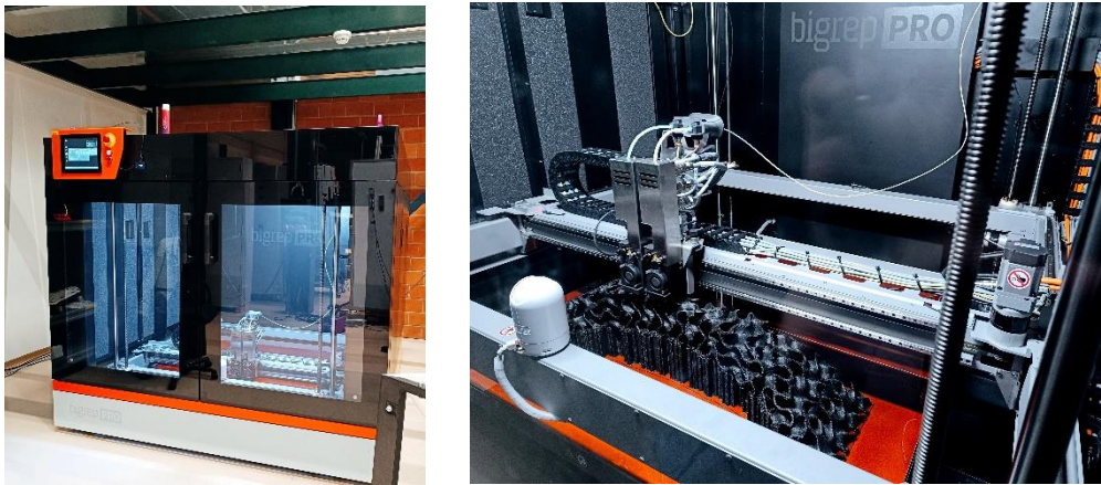
Figure 6.5 Bigrep PRO printer built print space of 1005 x 1005 x 1005 mm.
