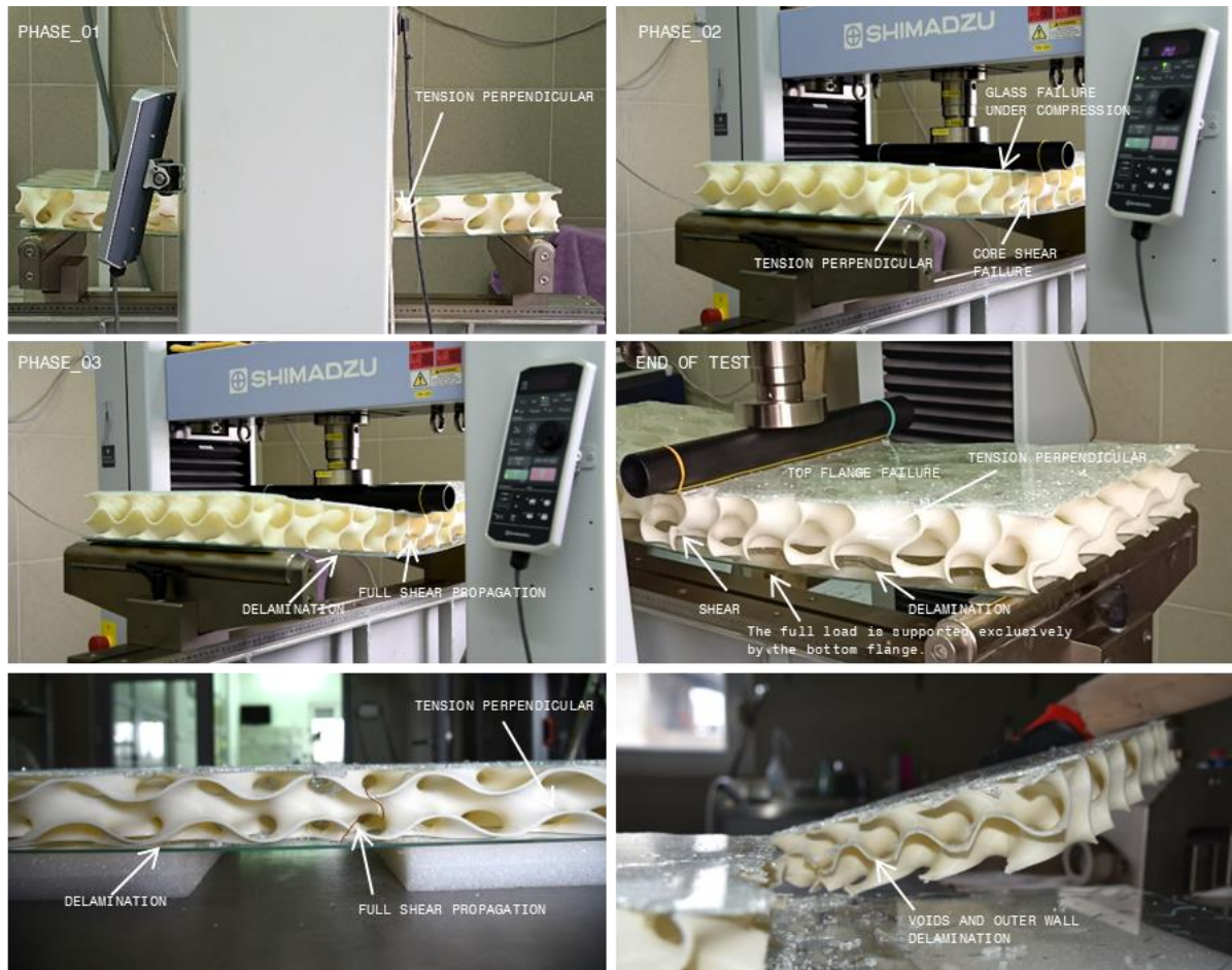
Figure 8.7 Snapshots from bending test by phases
