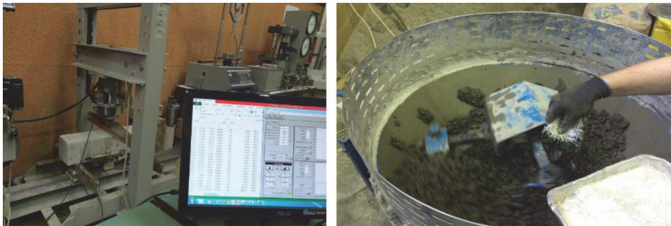
Figure 3. Preparation and examination of FRC specimens
