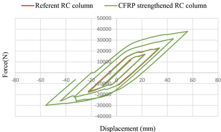
**Figure 4. Relation force-displacement**
