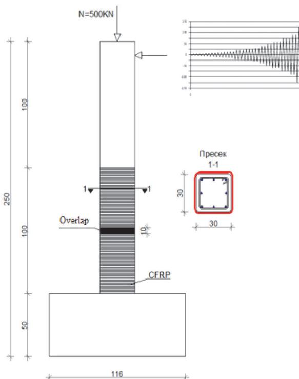
**Figure 2. Strengthened RC column subjected to cyclic loading**
