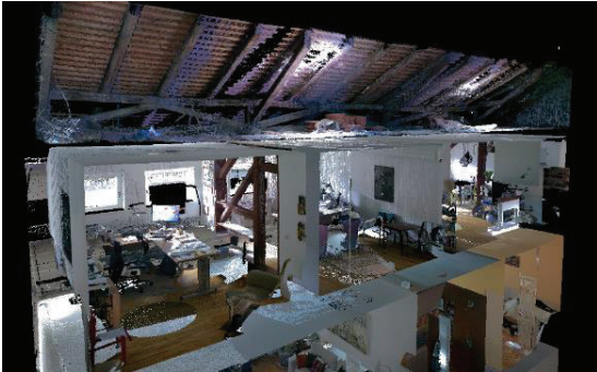
Figure 14: Point cloud of a case study building
