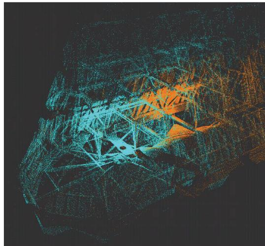
*Figure 18: Zagreb Cathedral – alignment of two scanning positions*
