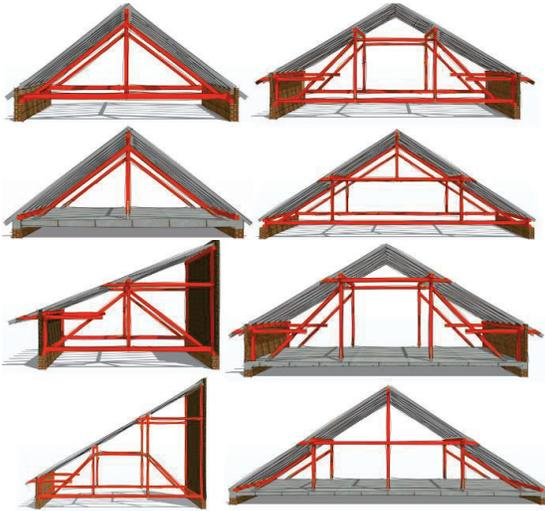
Figure 1: Typical timber roof structures in Zagreb
