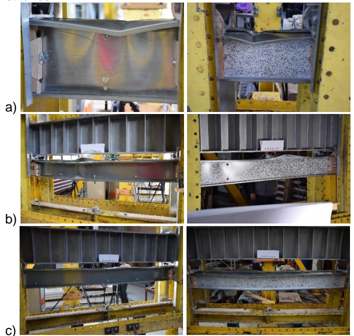
Figure 26: Deformations for 2C-St-B-240-2.0 a) Local, b) Distortional, c) Interactive buckling
