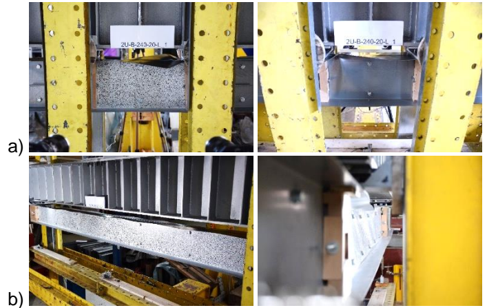
Figure 38: Deformations for 2U-B-240-2.0 a) Local, b) Interactive (Local+Global) buckling
