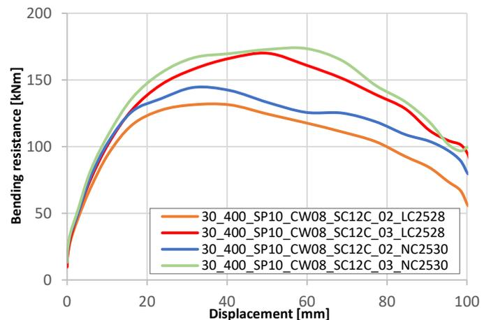
Figure 23: Influence of concrete type for shear connectors positioned in pairs
