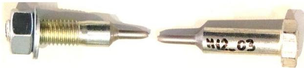
Figure 3: Tested specimen of the bolt as a demountable shear connector
