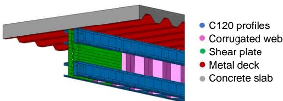
Figure 9: Floor system model in Abaqus/CAE
