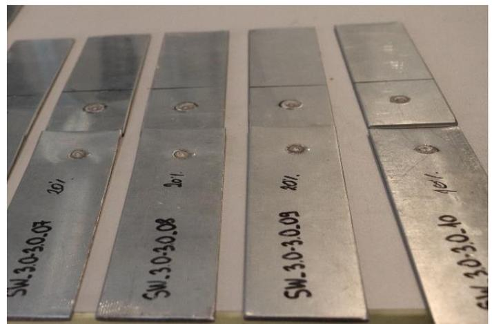
Figure 7: The interfacial fracture of the spot welds
