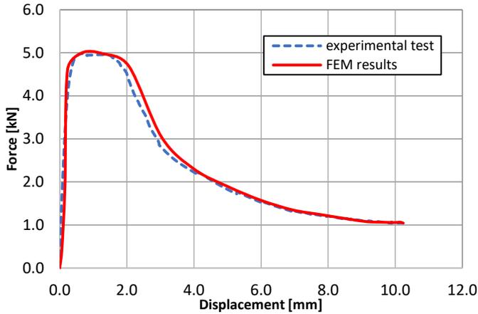
Figure 8: Spot weld testing for specimen SW 0.8-1.0
