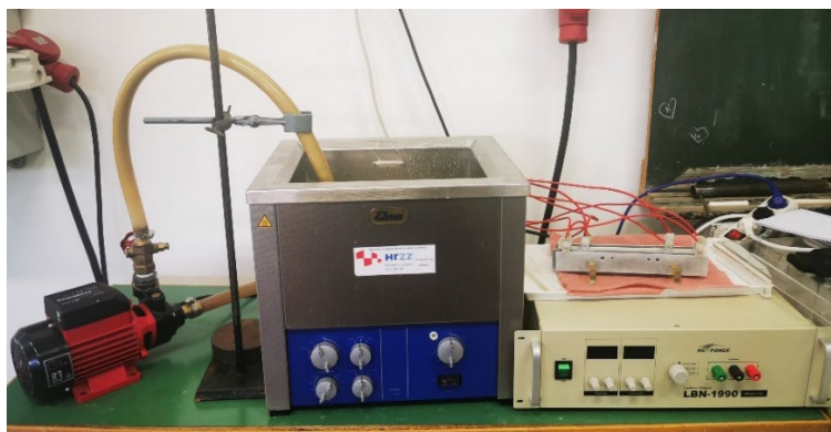
Figure 2. Modified ultrasonic bath with recirculation, laboratory power supply and aluminium electrodes
