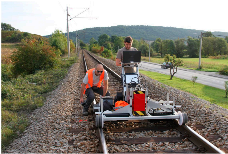
Figure 6. Conduction of GPR investigations.
