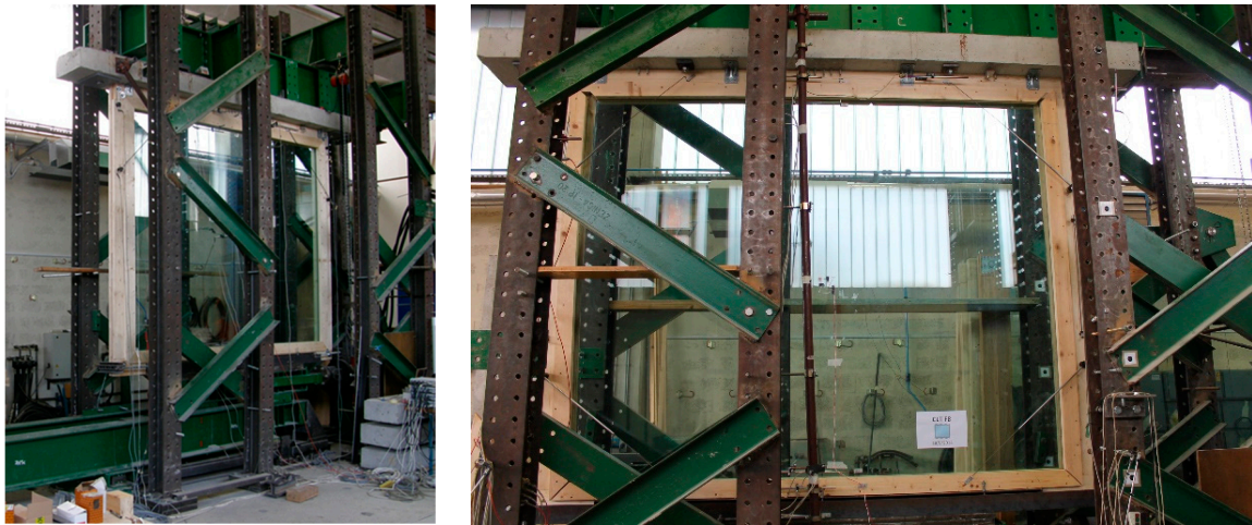
Figure 4. An example of a timber–glass composite system [39,40,88–94].
