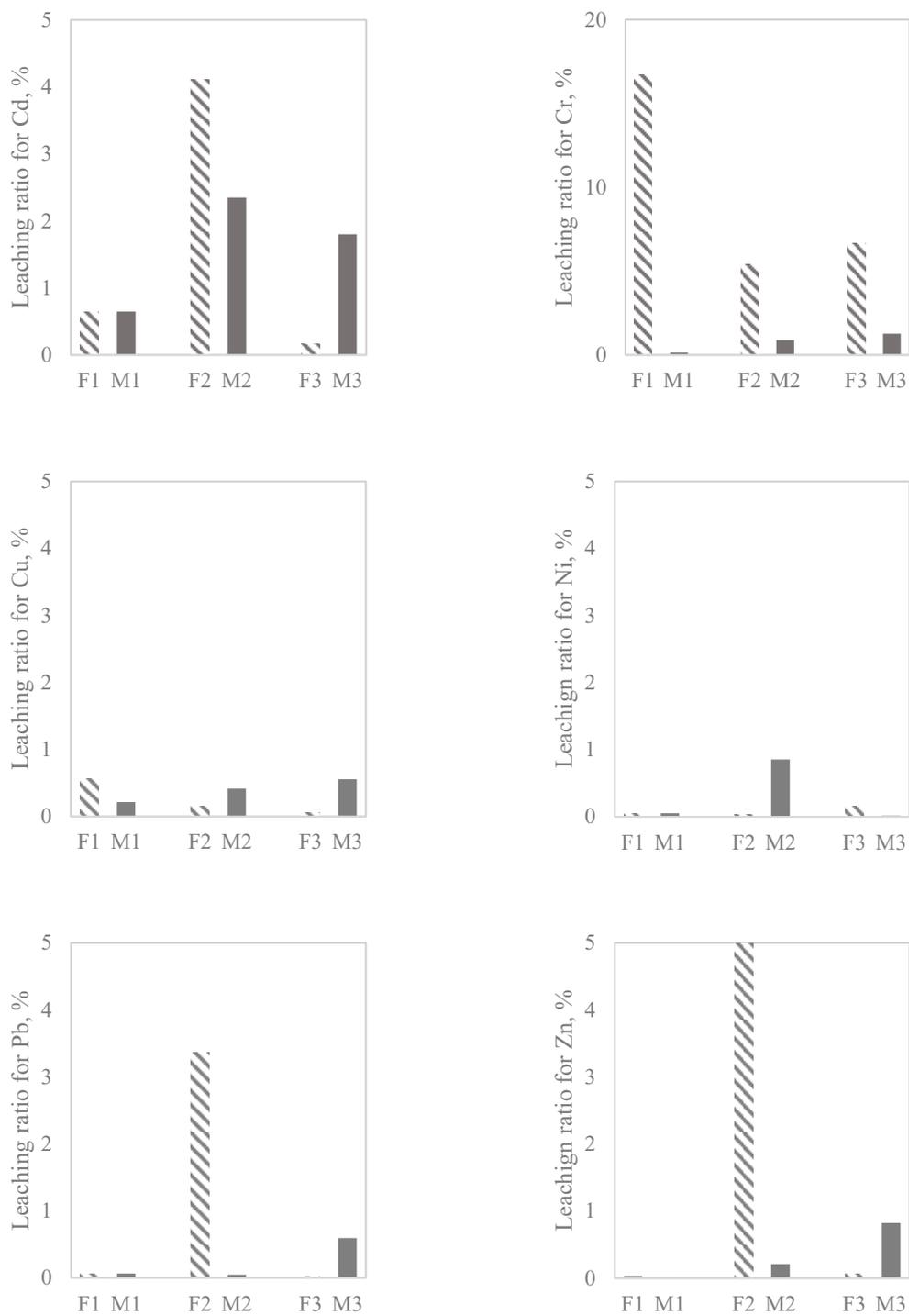
**Figure 1.** Ratio of leached metal in the crushed cement composite compared to the primary samples (WBA eluates F1, F2, and F3).
