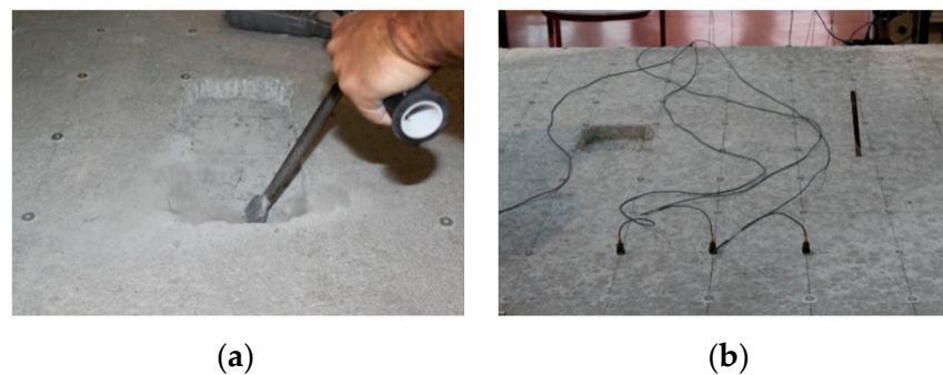
Figure 4. Discrete damages on the RC plate: (a) chiseling; (b) one of the damage locations on the concrete plate.
