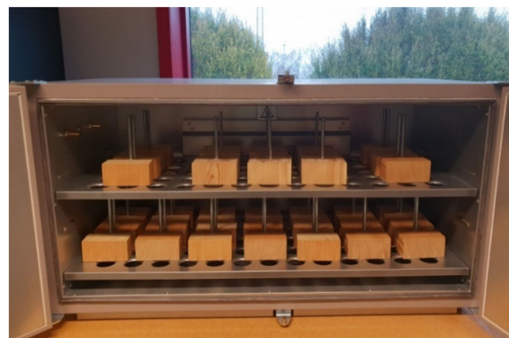
Figure 2. Preparation of specimens under controlled atmosphere.
