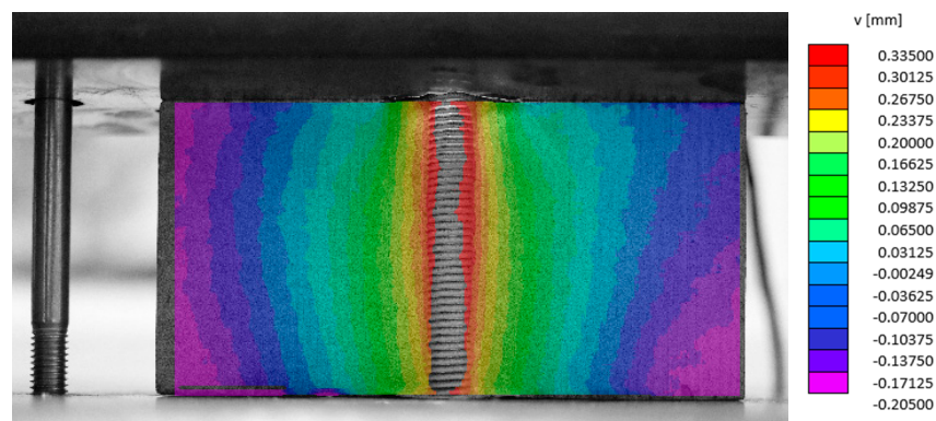
Figure 7. Example of the typical shear strain distribution along the rod, as obtained by digital image correlation (DIC).
