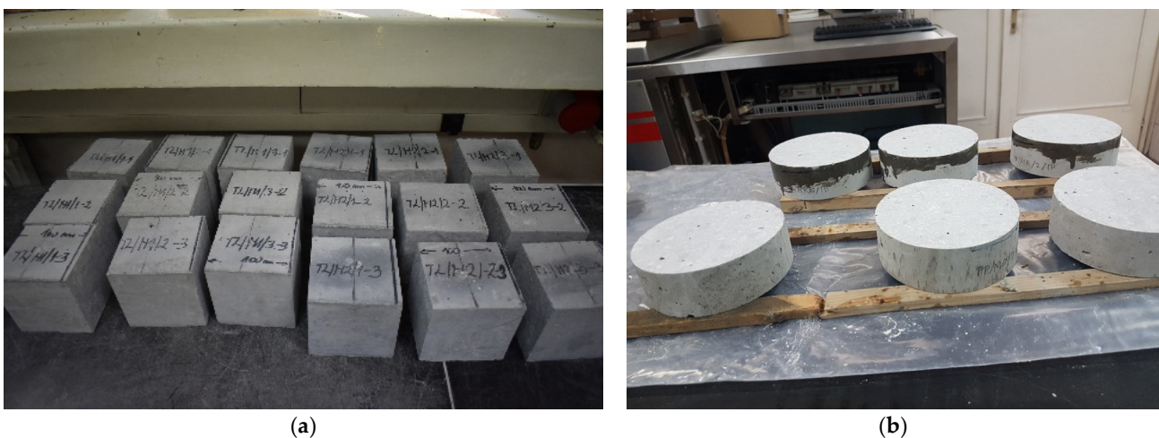
Figure 1. Preparation of samples for testing. (a) Cubes sawn from concrete prisms from the M1 and M2 mixes. (b) Coating of samples for capillary absorption measurement with epoxy resin.
