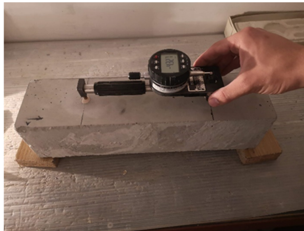
Figure 2. Measurement of the length change on the concrete prism.
