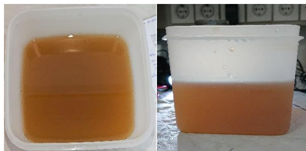
Figure 1. Initial solution in dark brown color containing 7.3 mg Mn/L.
