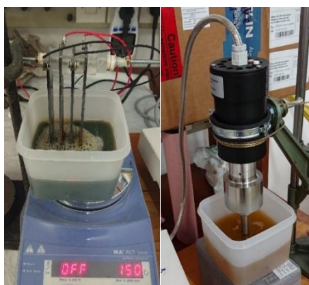
Figure 2. EC process with 4 Fe electrodes placed on a magnetic stirrer (left) and US homogenizer (right).
