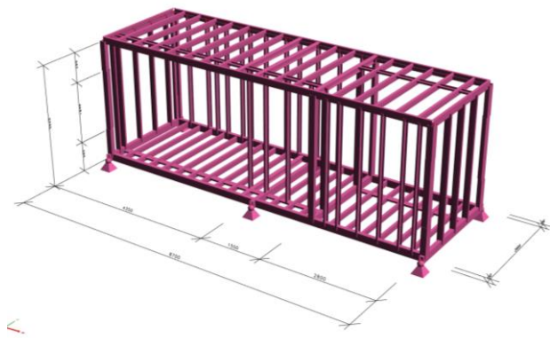
Figure 5. Load bearing steel structure of the MUZA: left —numerical model, right —realized structure.
