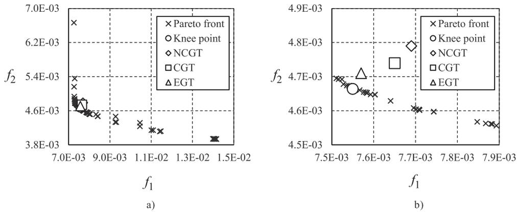
**Fig. 13.** a) comparison of the “knee” point obtained based on the pareto front (conventional method) with the position of the optimal solutions obtained using the three different game models (NCGT, CGT and EGT) b) detailed view of the position of the different solutions.
