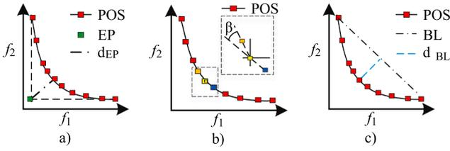
**Fig. 1.** Different methods to solve the decision-making problem (to find the optimal solution on the Pareto front): a) minimum distance from equilibrium point, b) maximum band angle, c) maximum distance from boundary line (Legend: POS - Pareto optimal solution; EP - Equilibrium Point;  $d_{EP}$  - distance from equilibrium point;  $\beta$  - band angle; BL - boundary line;  $d_{BL}$  - distance from boundary line).
