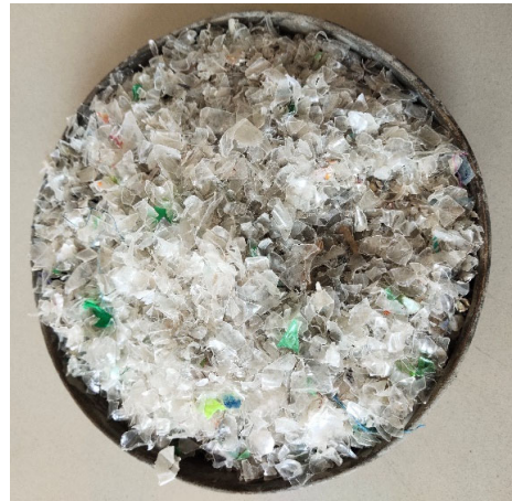
Figure 1. Crushed plastic waste of 4 mm to 5 mm in size.
