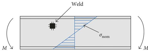
FIGURE 5: Nominal stress in a beam component.
