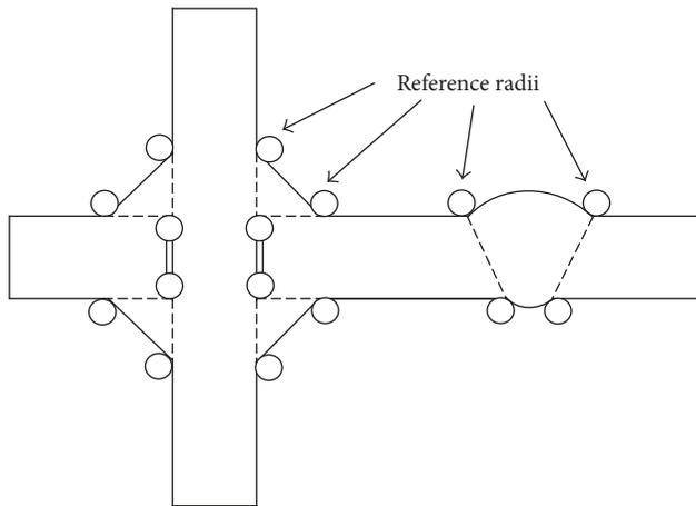
FIGURE 11: Stress evaluation in notch with referent radii.
