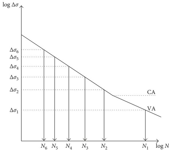
FIGURE 4: Palmgren–Miner hypothesis of linear damage accumulation.
