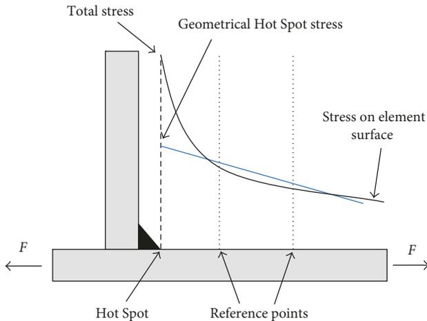
FIGURE 8: Definition of Hot Spot stress according to [25].
