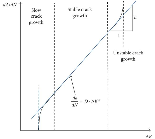
FIGURE 13: Typical curve of crack growth inside metals.
